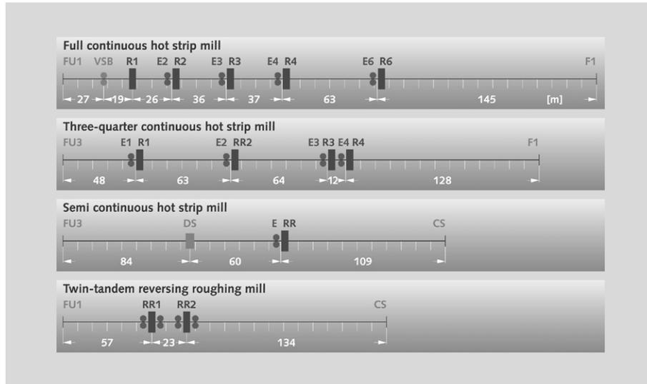
**Figure 10:** Layouts of hot strip roughing mills.
