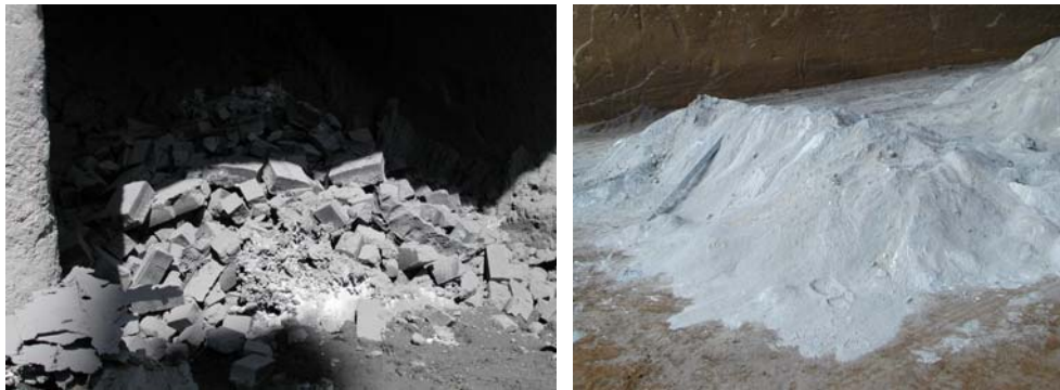
Figure 1. Examples of material that can be recycled: used refractory and ladle slag
