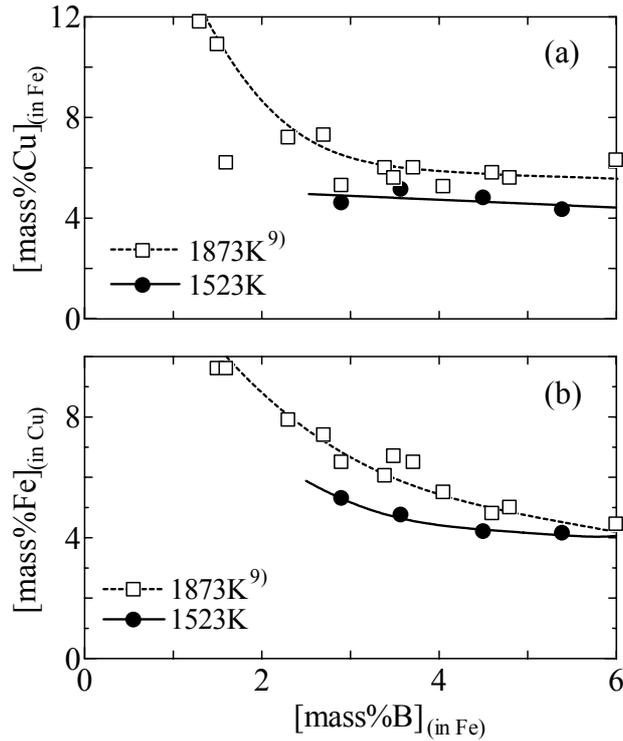
**Figure 2.** Effect of boron content of the Fe-rich phase on copper content of the Fe-rich phase and iron content of the Cu-rich phase.
