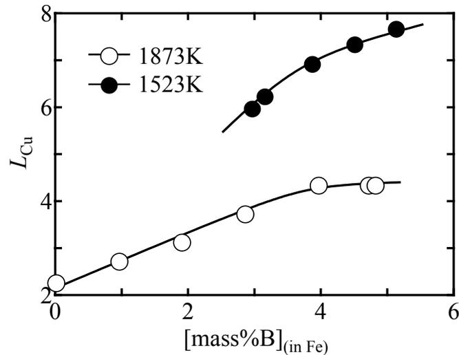
Figure 5. Effect of boron content of Fe-rich phase on  $L_{Cu}$ .
