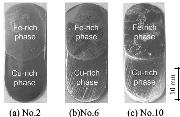
**Figure 1.** Images of separation into two liquid phases for several samples from Fe-Cu-B and Fe-Cu-B-C system (sample Nos. 2, 6 and 10).
