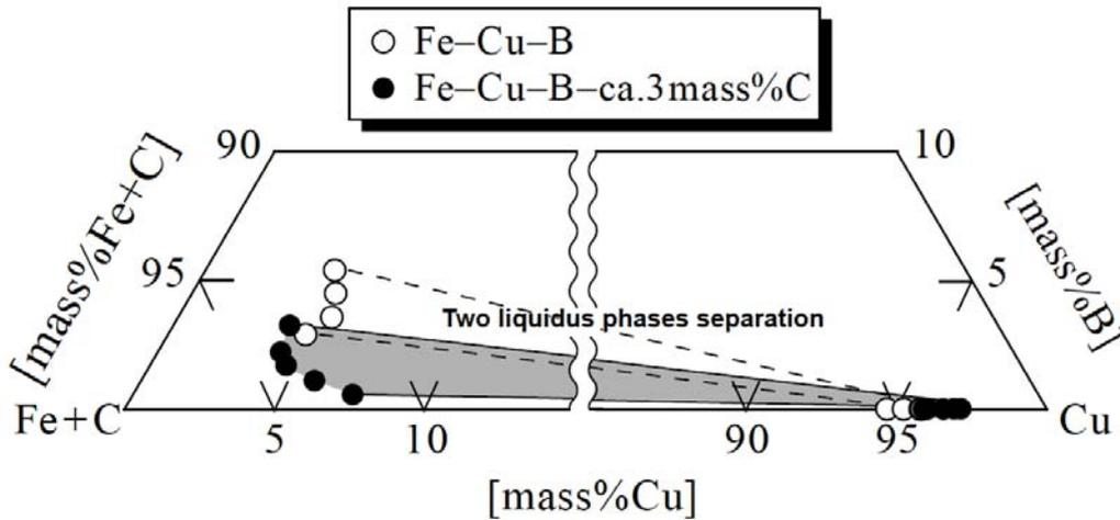
**Figure 4.** Region of two liquid phases for Fe-Cu-B-C system at 1523 K.
