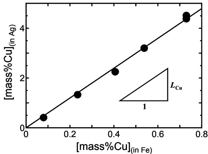
Figure 6. Relationship between copper content of Fe-rich and Ag-rich phases at 1523K. ( $[\text{mass}\%B]_{(\text{in Fe})}=3$ )
