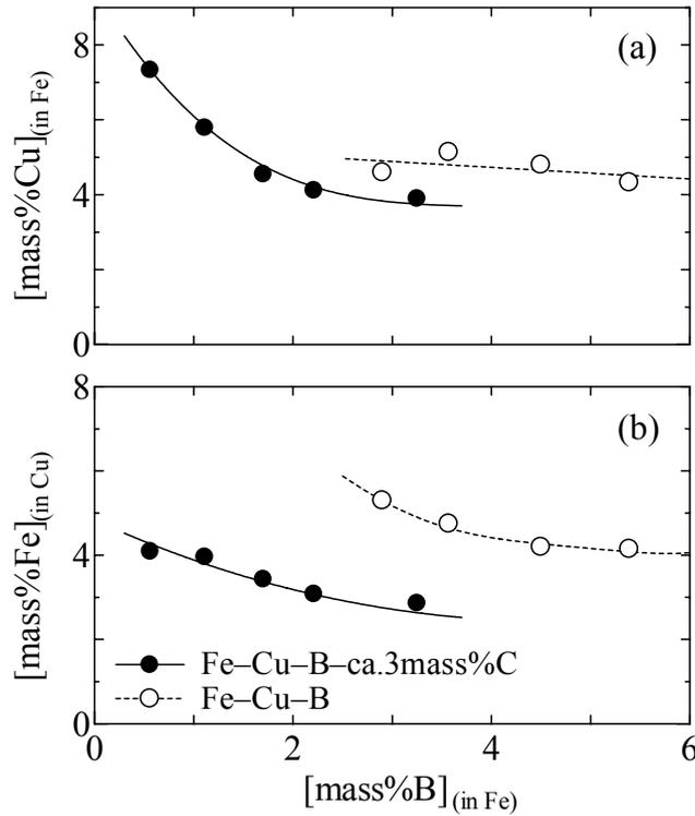
**Figure 3.** Effect of boron content of the Fe-rich phase on copper content of the Fe-rich phase and iron content of the Cu-rich phase at 1523 K.
