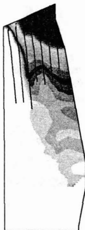
Figure 18 : Example of temperature distribution (mullet points probing)
