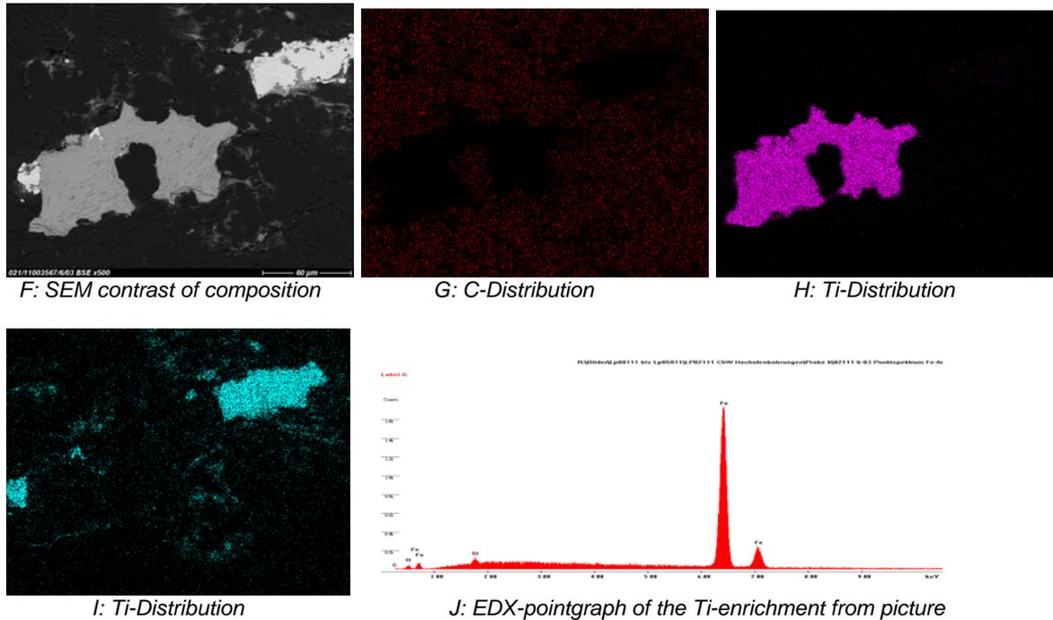
**Figure 11.** Investigation of the sample Section 6 bottom n° 5.
