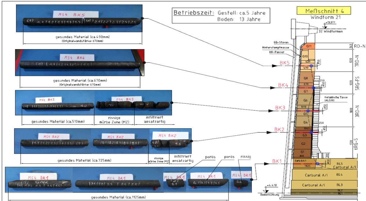
Figure 7. Core boring samples from the hearth walls.
