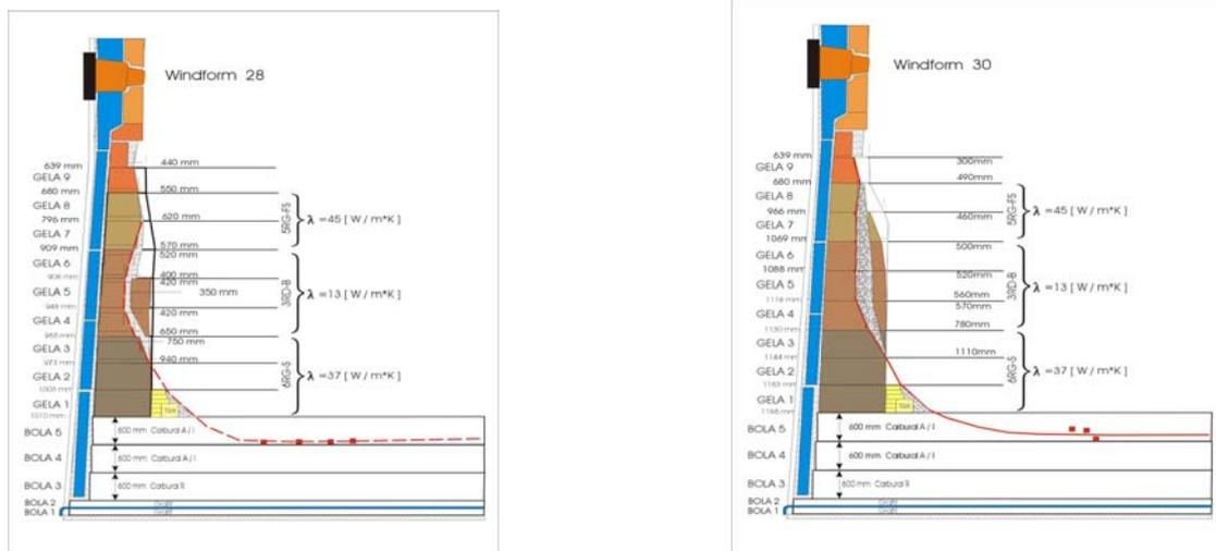
**Figure 4.** Measurements of the wear of the hearth walls.
