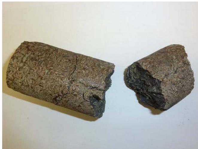
**Figure 10.** Core boring sample section 6 from bottom layer inside.
