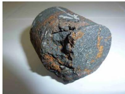
Figure 8. Core boring sample from hearth level 5 inside.
