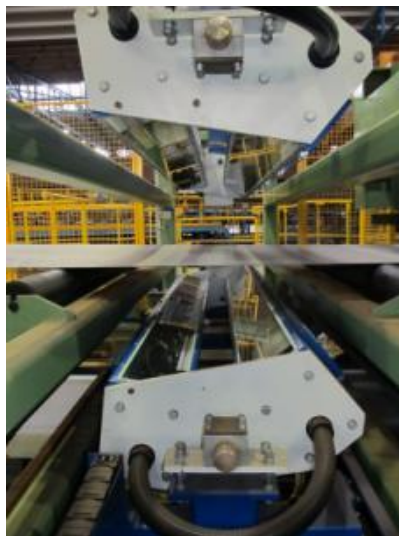
Figure 8. Compact surface inspection sensor for top and bottom strip inspection.
