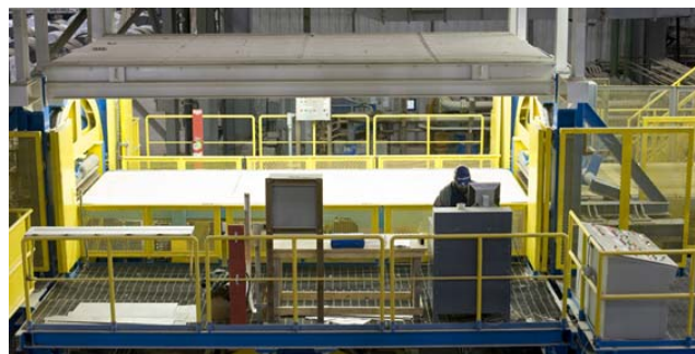
Figure 7: In-line inspection "Rotary Inspect".
