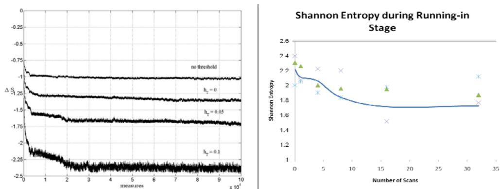
**Figure 4.** An example of decreasing Shannon entropy with time during the transient process [2] experimental results for WC pin vs. Cu disk UHV tests.
