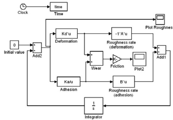
**Figure 2.** A feedback loop model in Simulink Two simultaneous processes (adhesion and deformation) affect surface roughness in different manners. Consequently, an equilibrium value of roughness exists, which corresponds to minimum friction.
