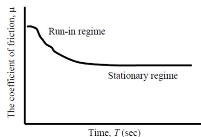
**Figure 1.** Typical decrease of friction during the running-in
