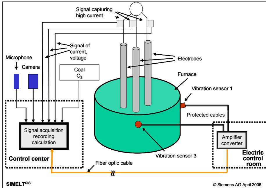
Figure 2. Measurement system
