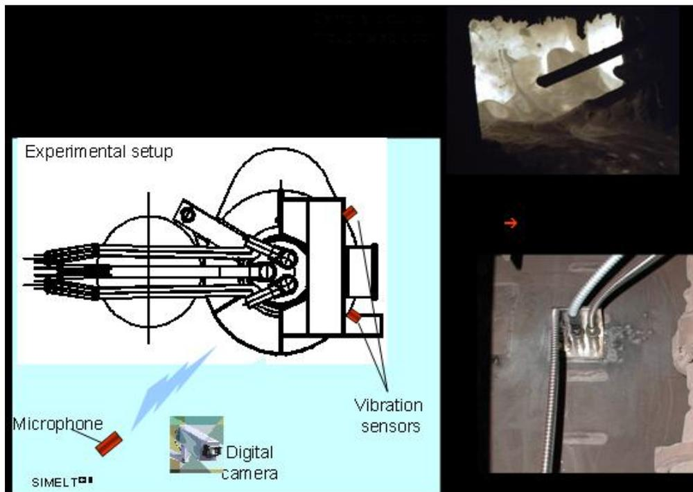
**Figure 1.** Experimental setup: vibration sensors, camera and microphone
