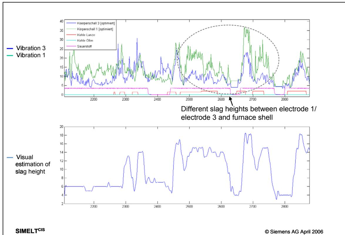
**Figure 7.** Spatial variation inside the furnace: comparison of sensors close to electrode 1 / electrode 3 (heat #219229)
