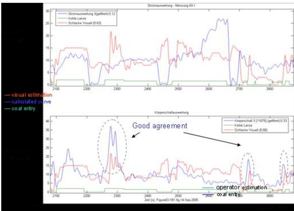
Figure 6. Comparison between current and vibration analysis: heat #219266
