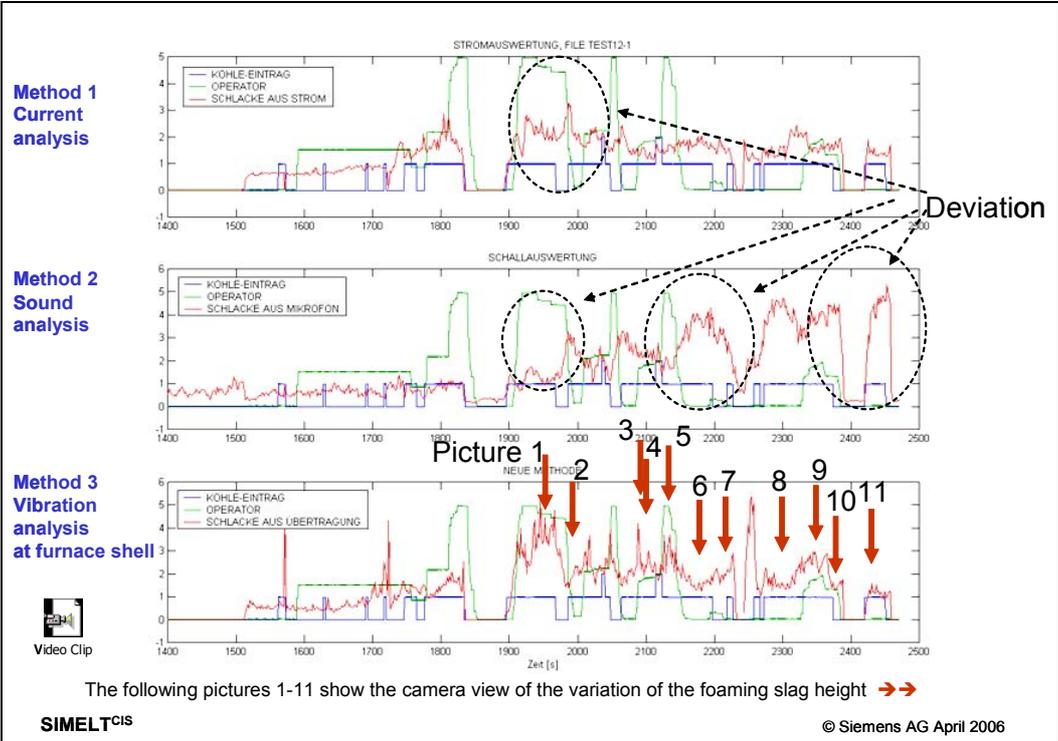
**Figure 4.** Comparison of methods for one example: foamy slag phase
