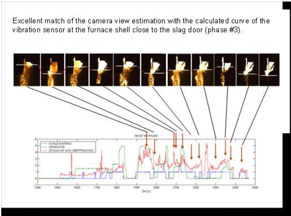
Figure 5. Comparison of the camera view with calculated curve
