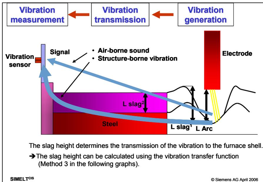
Figure 3. Principle of vibration evaluation
