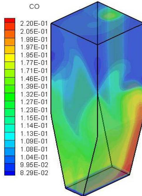
Figure 7. CO percentage distribution in fluidized bed reactor.
