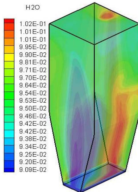
Figure 5. Percentage Distribution of water steam in fluidized bed reactor
