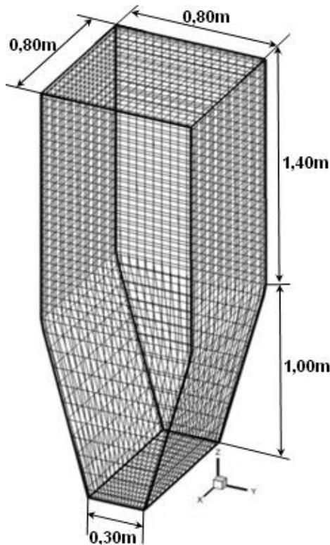
Figure 2. Mesh generated by volume finite method.
