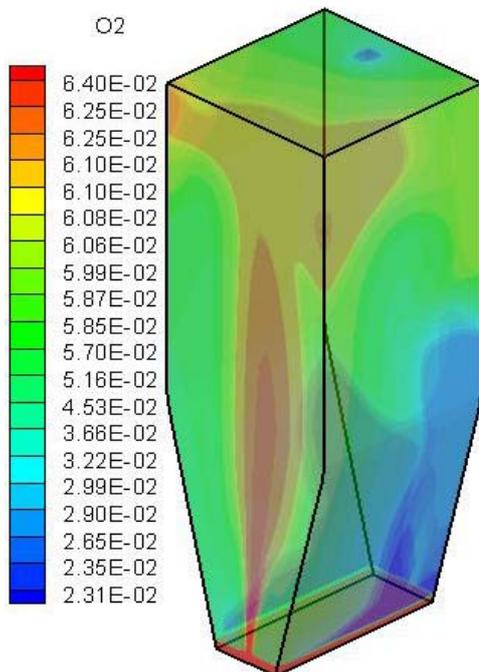
Figure 4. O<sub>2</sub> percentage distribution in fluidized bed reactor.
