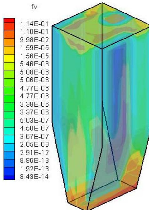
**Figure 9.** Coal behavior in the fluidized bed reactor.
