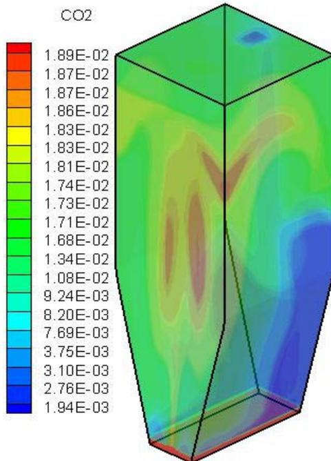
Figure 6. CO<sub>2</sub> percentage distribution in fluidized bed reactor.
