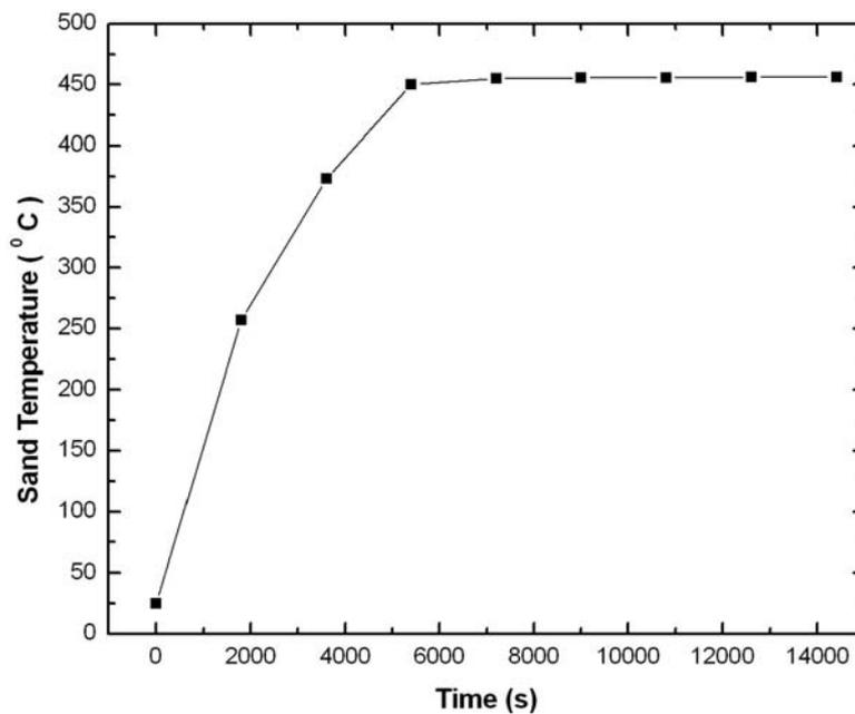
Figure 3. Curve of heating of fluidized bed reactor obtained by simulation.
