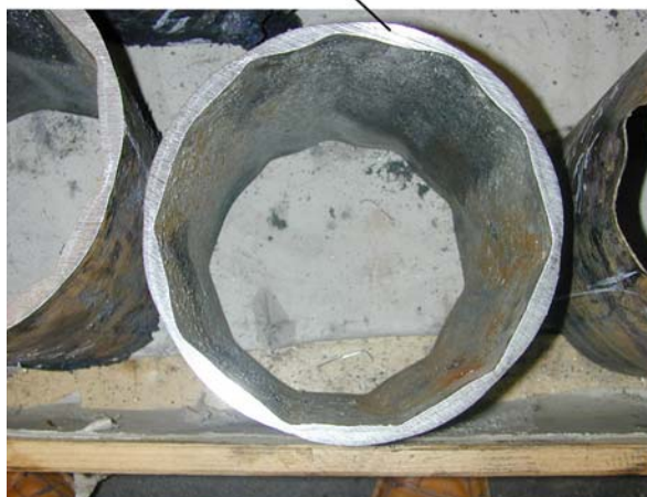
Figure 10. Real break out strand shell of a peritectic steel grade.
