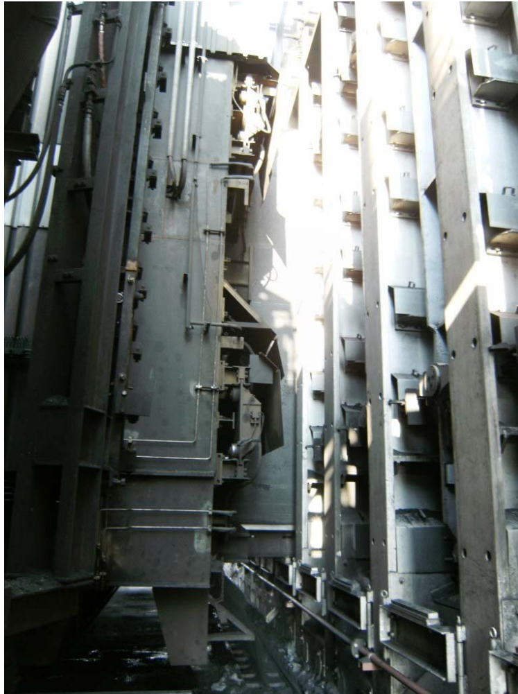
Figure 2. Charging a coal cake with stamp charging technology.
