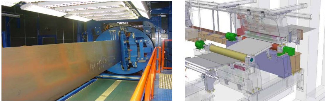
Figure 8. Inline strip inspection systems in the continuous exit module (automatic type in the right picture)
