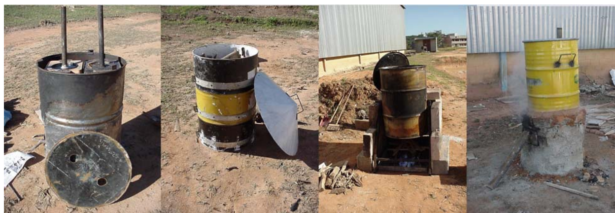
Figure 5. Prototypes charcoal kilns for granulated material.
