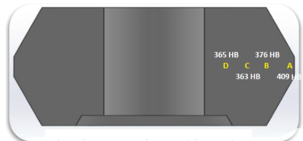
Figure 9. Brinell results from the surface down to the core.
