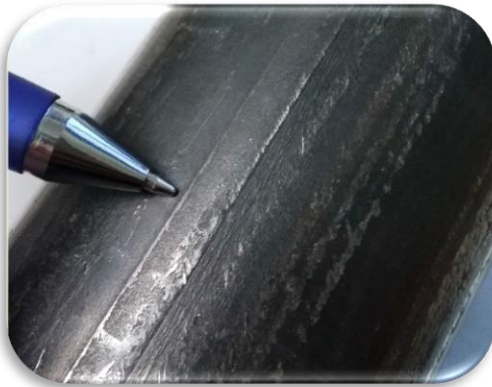
Figure 1. External longitudinal marks on a tube surface with OD 1 ¼”.
