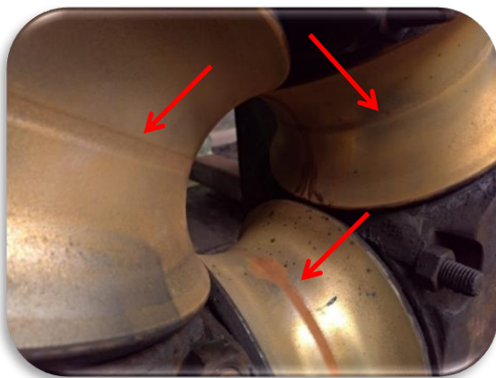
Figure 2. Representation of wear on rolls surface.
