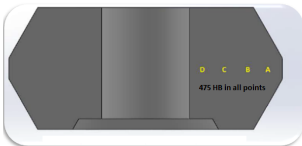
Figure 13. Brinell results from the surface down to the core in a quenched and tempered roll.
