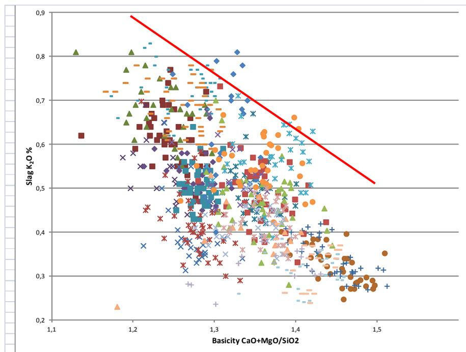
**Figure 4.** Slag  $K_2O$  content for various furnaces, monthly averages. The red line shows the assumed maximum slag  $K_2O$ % for basicity  $((CaO+MgO)/SiO_2)$  in the range 1,25-1,45 in our model.
