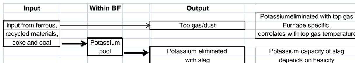
Figure 3. Outline of a simple model for elimination of potassium from a blast furnace.
