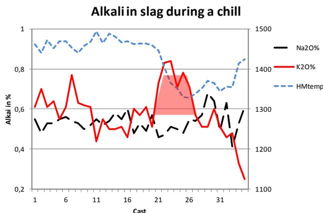
Figure 1. Slag K<sub>2</sub>O and Na<sub>2</sub>O % during a chilled furnace condition. The x-axis covers about 4 days.
