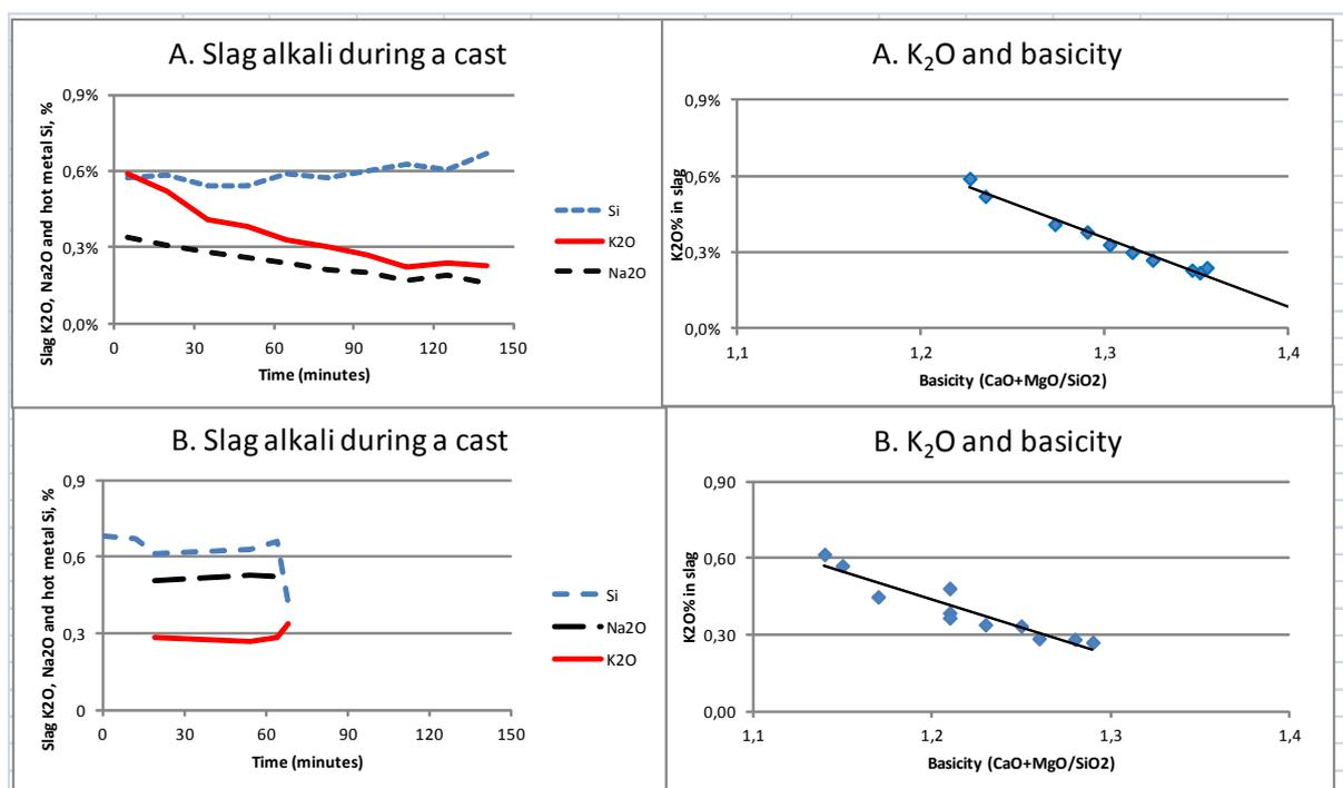
Figure 2. Slag K<sub>2</sub>O % during a cast and the correlation between basicity B3 and K<sub>2</sub>O % during a cast. A: Ternium Siderar BF2, B: CAP/CSH BF1.
