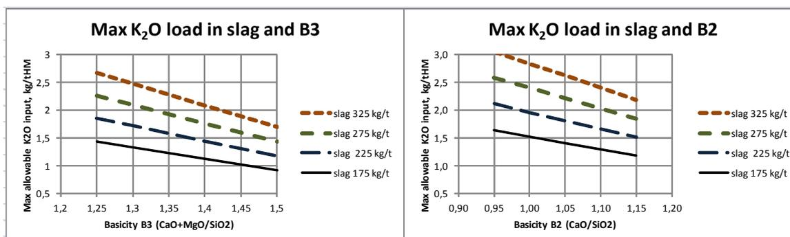
**Figure 6.** The maximum allowable K<sub>2</sub>O input (monthly average) assuming no elimination of K<sub>2</sub>O via the top for different slag basicity and slag rates. At the left hand side a graph based on 3-component basicity, on the right hand 2-component basicity. Slag rates are indicated on the right side of the graphs. For details see text.
