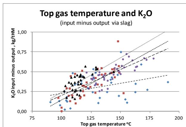
**Figure 5.**  $K_2O$  removed with top gas (in kg/tHM) as a function of top gas temperature. The figure shows monthly averages for the difference between  $K_2O$  input and output via slag for four different furnaces and linear regression lines for the four furnaces.
