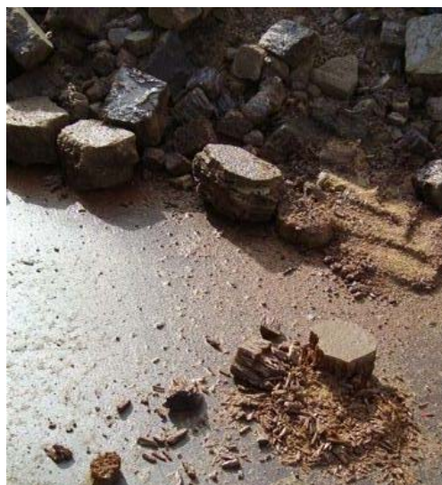
Figure 6. Stretford low quality Sulphur (Solidified Product after Autoclave).
