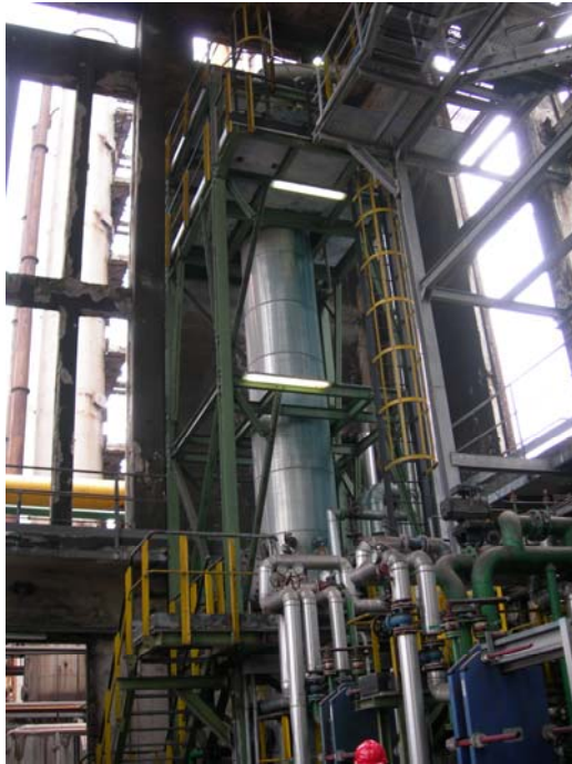
Figure 10. Titanium made NH 3 / H 2 S stripper for high efficiency removal
