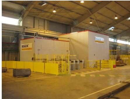
Figure 14. Grinding machine, type HP 6, for Titanium ingots and slabs
