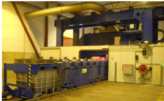
Figure 9. Gantry-type abrasive cut-off machine of special design, type TS 20 FPS for hot cutting of round, squared and flat forgings coming from an open-die forging press
