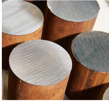
Figure 2. Cold cut product ends Figure 3. Hot cut product end
