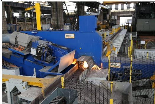
Figure 5. BRAUN abrasive cut-off machine, type TS 20 L (2.000 mm cutting wheel dia.) for hot cutting of forged bars
