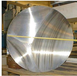
Figure 7. Workpiece with 915 mm diameter after index cutting
