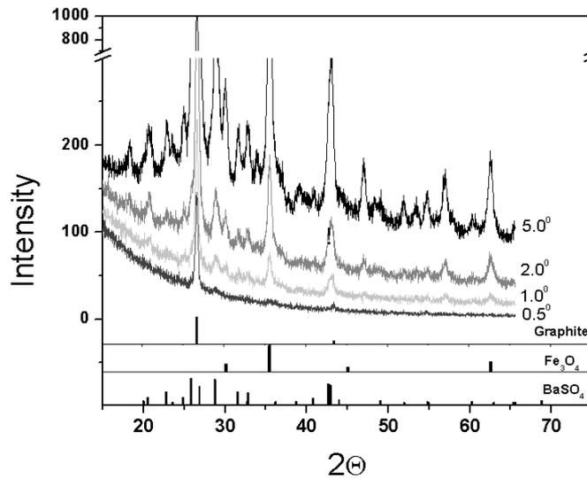
**Figure 5.** GIXRD patterns of PMC pad, showing different peaks for different penetration depths. Peaks of most important phases are indicated below.
