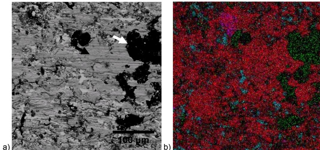
**Figure 1.** Friction film on a PMC pad; a) BEI, grey striated areas (black arrow) are the third body, dark contrasts indicate low Z elements (white arrow); b) composite map of selected elements (Fe red, C green, Ba cyan, Si magenta). Scale bar 100 μm.
