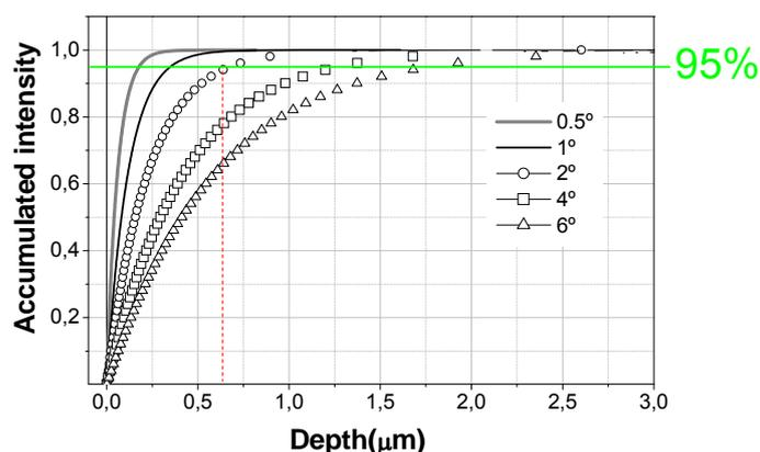
**Figure 4.** Cumulative diffracted intensity as a function of sample depth. The incidence angles are indicated on the image label. The intercept of the curves with the green 95% line indicates the probed sample depth, e.g. the red drop line on the intercept with the 2° line indicates a probed thickness of 0.7  $\mu\text{m}$  when measuring with 2° incidence).
