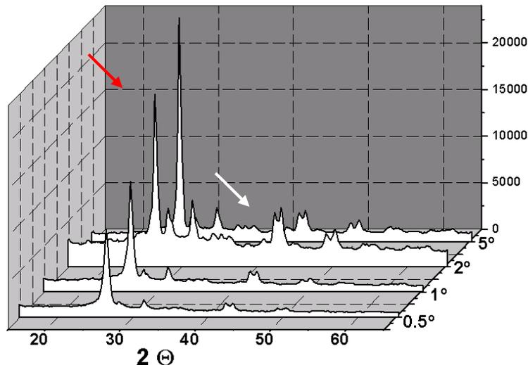
**Figure 6.** GIXRD patterns of PMC pad, showing different depth evolution of graphite (red arrow) and barite (white arrow).
