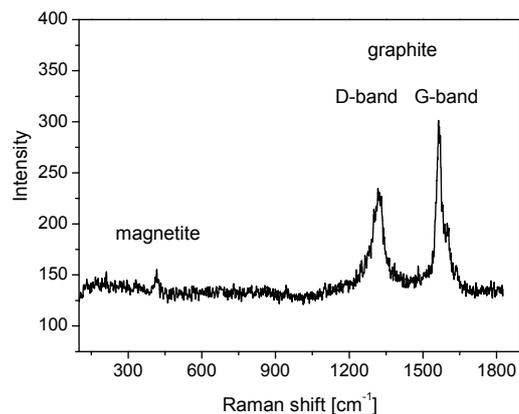
**Figure 2.** Typical micro-Raman spectrum from a friction film. Magnetite peak and graphite D- and G-bands are indicated.
