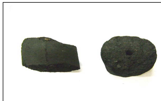
Figure 1b – Briquette containing 3% of charcoal fines and 2% of rice hull coal
