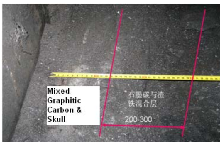
Figure 2. Mixed graphitic carbon powder and skull on hot face of carbon block of China’s Meishan No.3 BF hearth.
