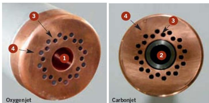
**Figure 5** - Oxygenjet and Carbonjet tip design: 1-oxygen, lance phase, 2-carbon, 3-fuel, 4-oxygen, burner phase.
