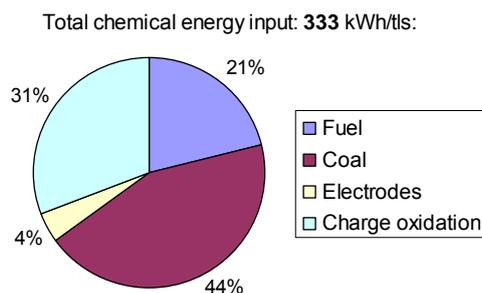
Figure 9 - Chemical energy sources (heats 100-190, after start-up).
