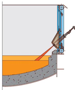
Figure 4 - Oxygenjet installed on a water-cooled, copper bulged panel.
