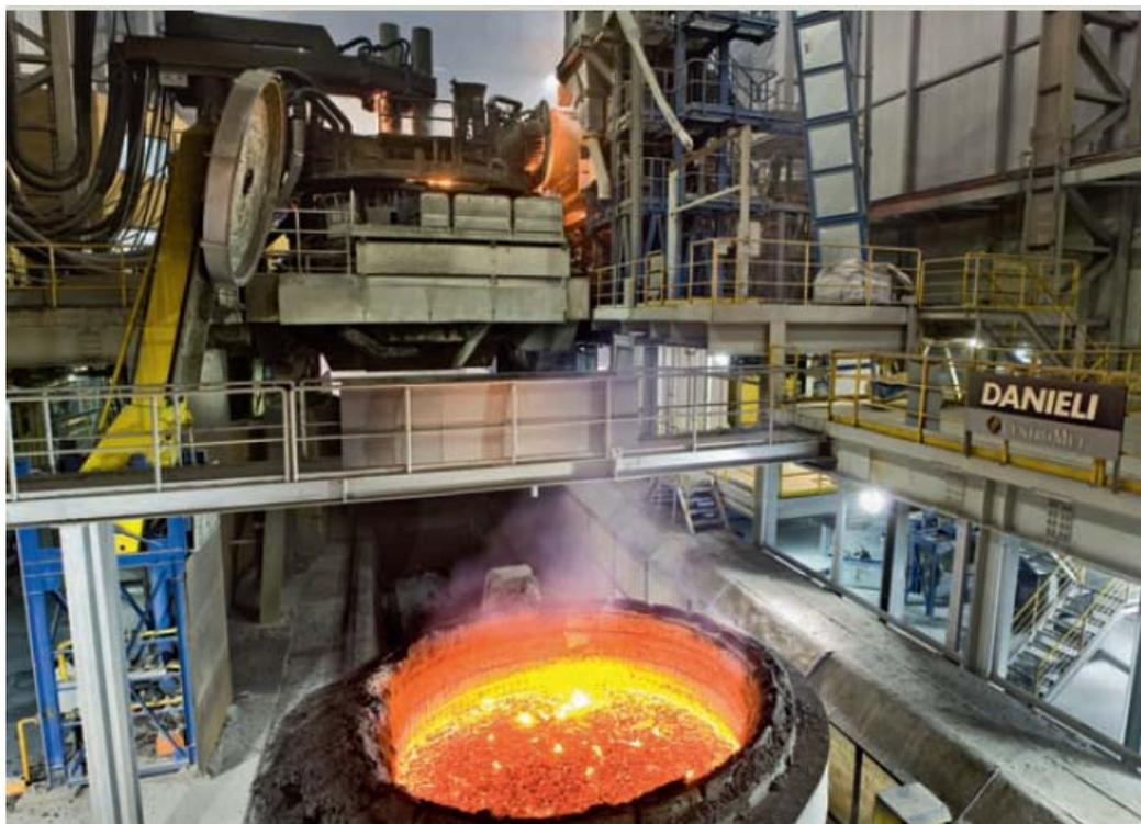
**Figure 1** - Kosco 100-t Fastarc AC electric arc furnace and ladle ready to be transferred to the steel refining station.
