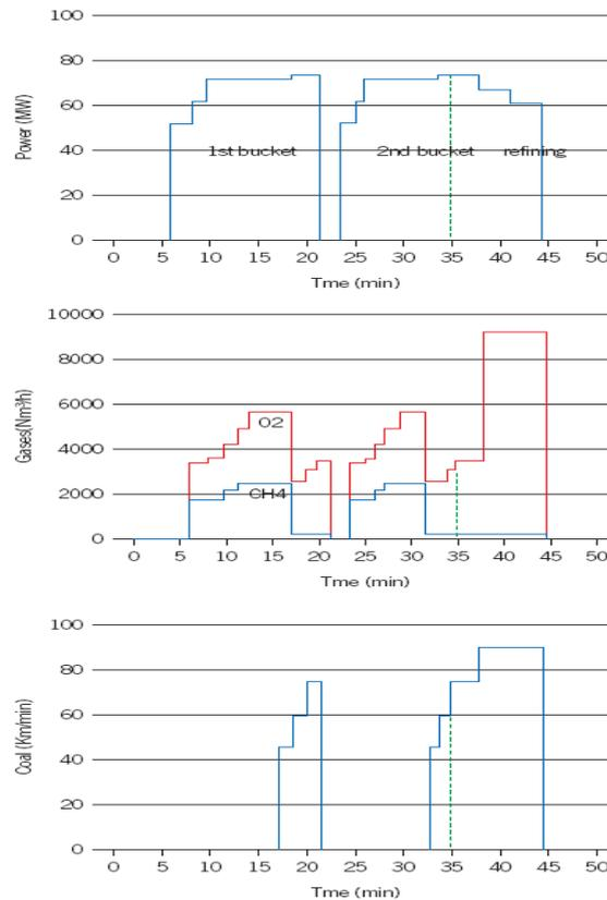
**Figure 6** - Melting profile showing active power input and alternative energy input.
