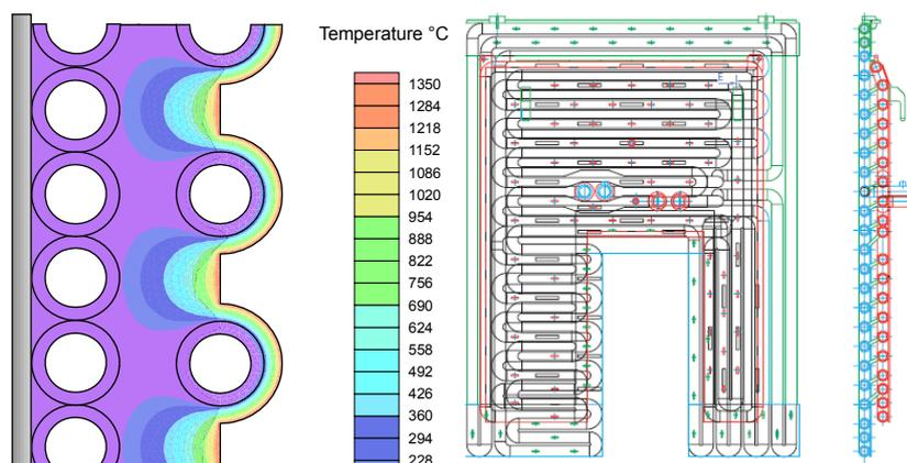
**Figure 2 – Energy saving panels: design and temperature gradients.**
