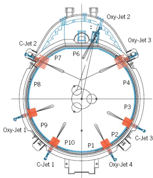
Figure 3 - Injection modules layout.
