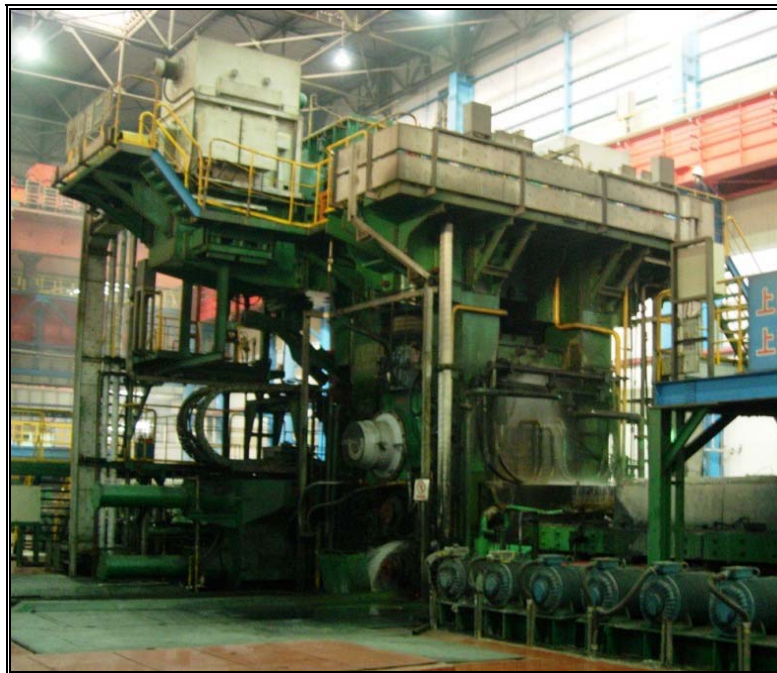
Figure 3 – Roughing Mill stand with attached Vertical Edger
