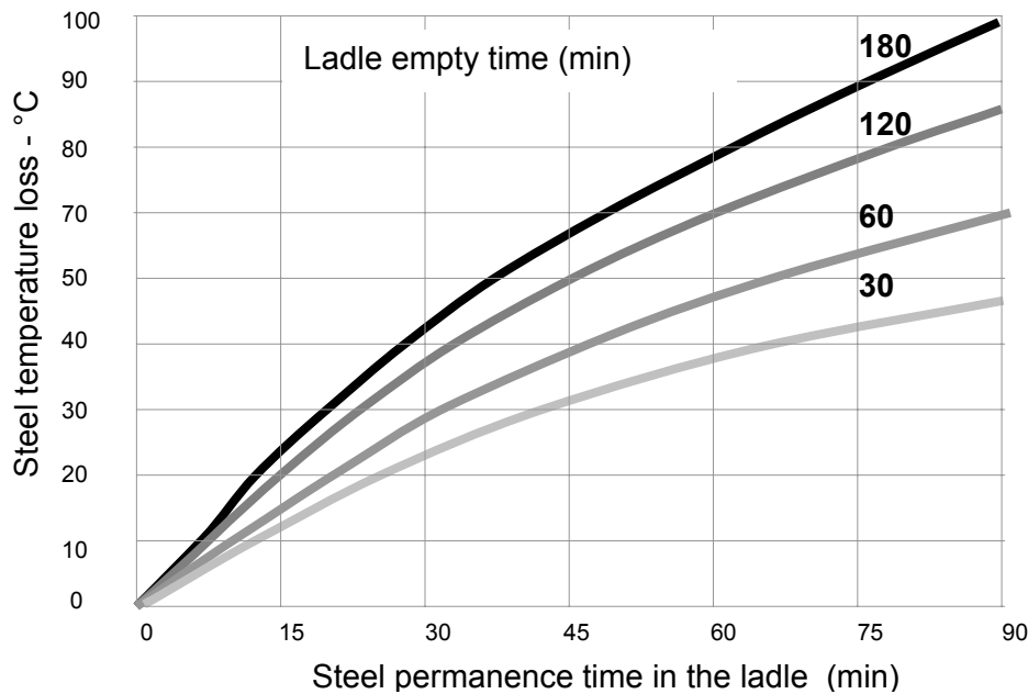
Figure 7. Temperature loss in steel depending on different ladle empty times.
