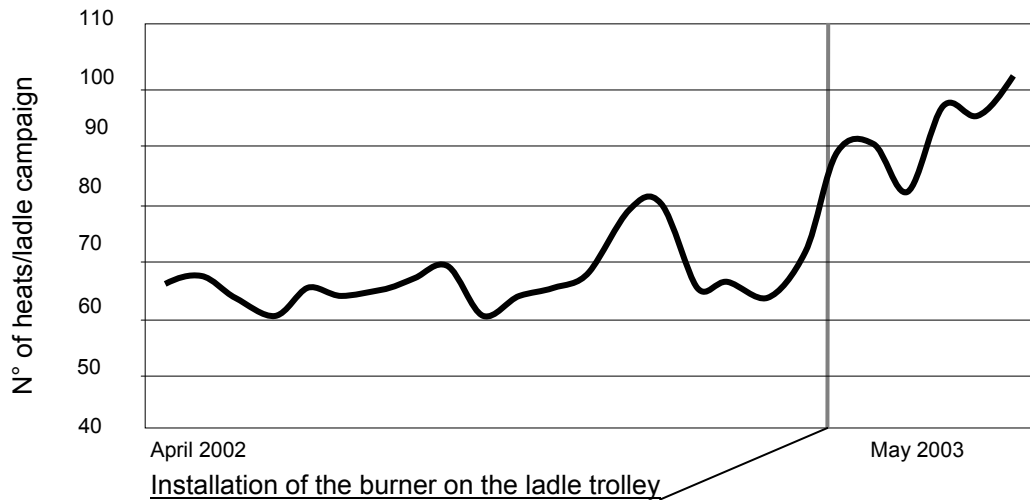
Figure 9. Development of the refractory performance of a Dolomite ladle lining in an EAF Steelplant
