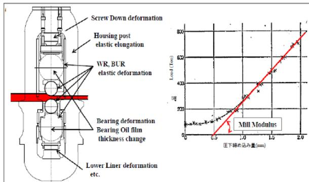
Figure 11: main components affecting the Stand mil modulus.
