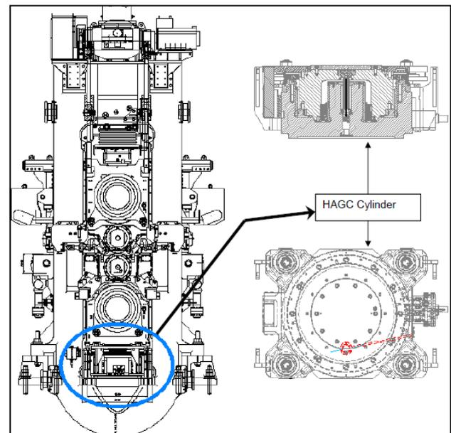
Figure 8: drawing with the positioning of the hydraulic capsules on the base of the stand mill
