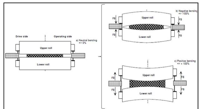
Figure 5: Bending actions to control the crown.
