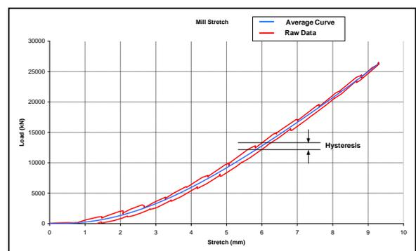
Figure 13: Example of a hysteresis curve.
