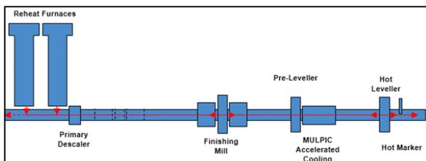
Figure 1: Layout of the Mill Area and main equipment.
