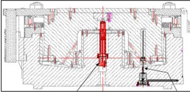
Figure 9: Positioning of the transducers in the hydraulic capsule.
