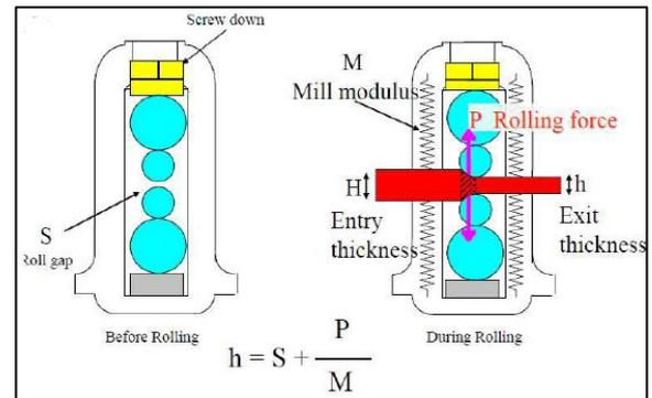
Figure 12: Example of the change in the mill modulus during a rolling.
