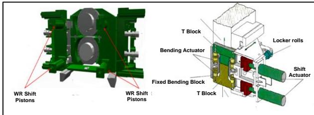
Figure 6: Work Roll Bending and Work Roll Shifting arrangement with Smart Crown.
