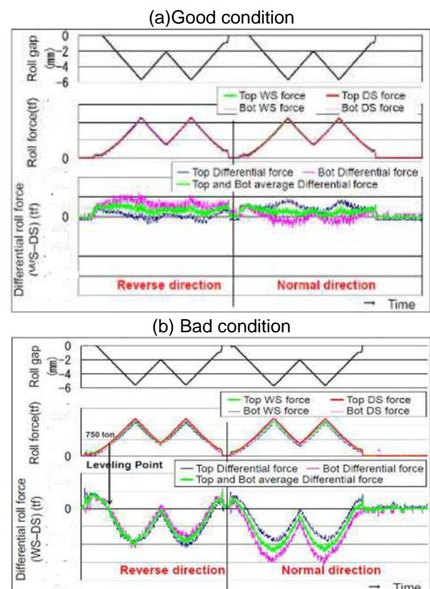
Figure 10: examples of good and bad conditions of the cross rolls.
