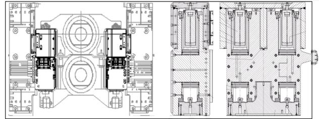
Figure 4: Frontal and lateral view of the Bending block location in the stand mill.
