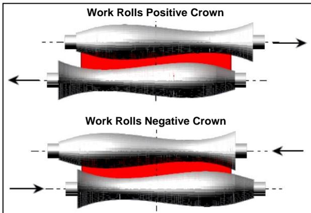
Figure 7: Basic principle of the work rolls profile for use in the Smart Crown.
