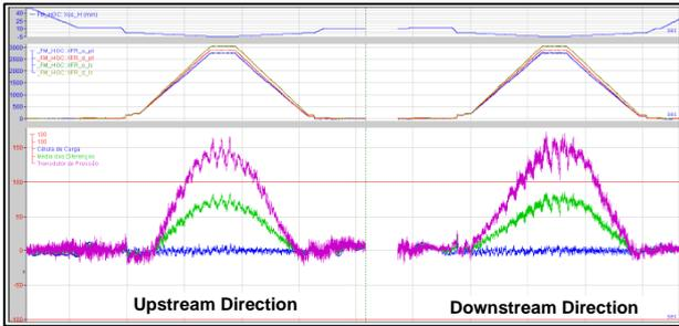
Figure 17: Crossover test with a non-expected performance.
