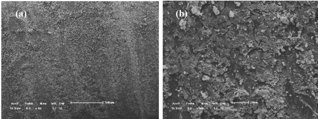
Figure 7. SEM fractographs of a pure polyester sample with different magnifications: (a) 40x, and (b) 500x.
