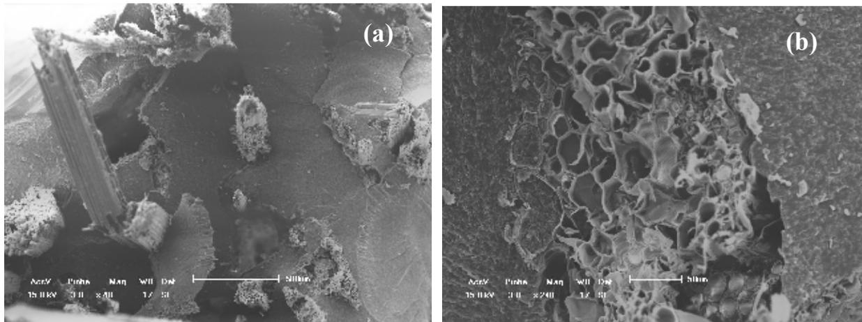
Figure 8. SEM fractographs of a 30% thinner buriti petiole fiber reinforce composite with different magnification: (a) 40x, and (b) 240x.
