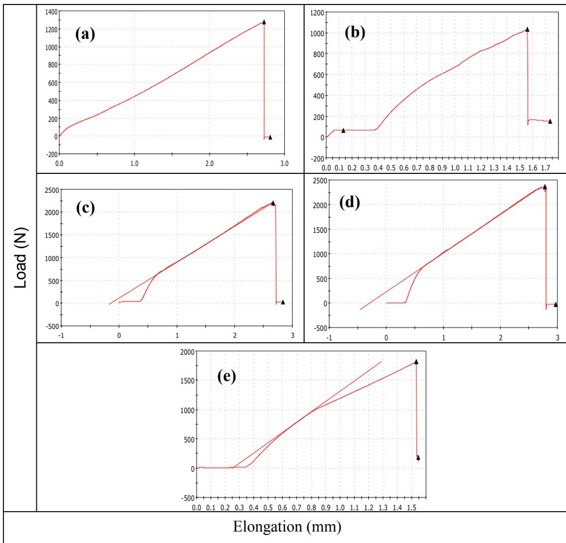
Figure 3. Tensile load vs. elongation curves for polyester composites reinforced with: (a) 0%, (b) 10%, (c) 20%, (d) 30%, and (e) 40% of volume fraction of thinner buriti petiole fibers.
