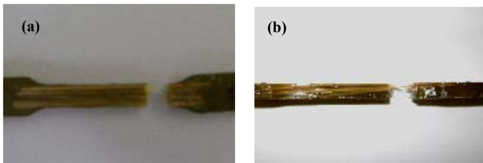
Figure 6. Macroscopic aspect of the ruptured tip of a polyester composite specimen reinforced with 40% of thinner buriti petiole fibers. (a) front view; (b) side view.
