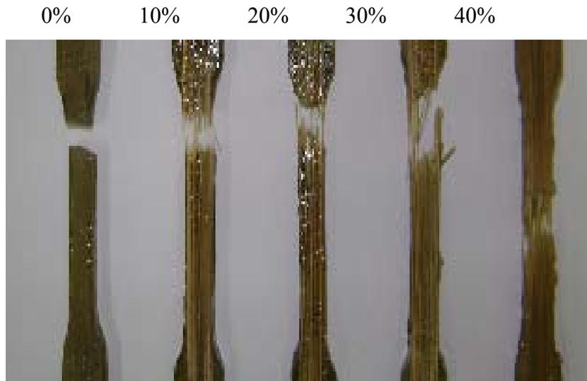
Figure 4. Representative tensile-ruptured specimens corresponding to the different volume fraction of thinner buriti petiole fiber in the polyester composites.
