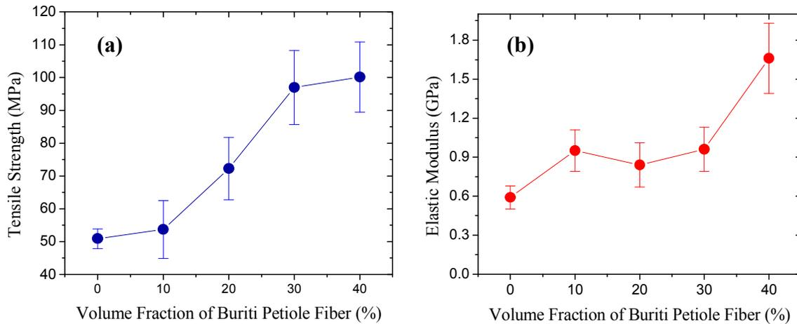
Figure 5. Variation of the tensile strength (a) and the elastic modulus (b) with buriti petiole fiber reinforced polyester composites.
