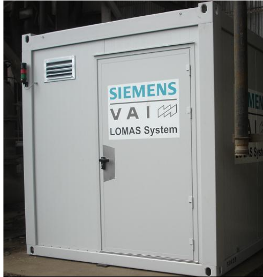
Figure 5. Lomas container including off-gas cleaning, preparation and analyzing technology.
