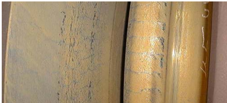
Figure 6. Fire cracks rolling rails, (5)
