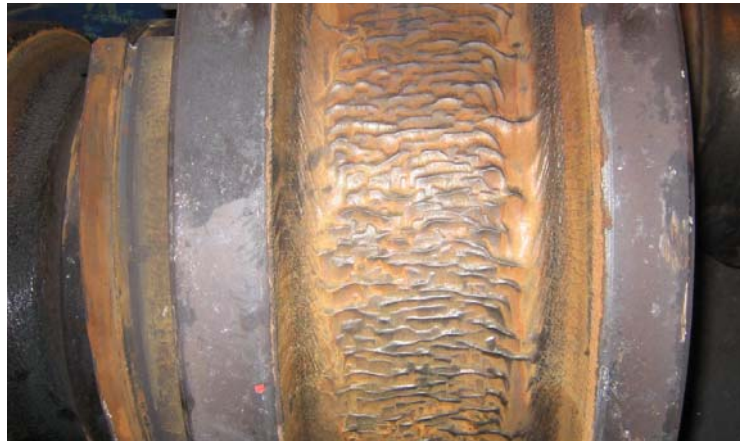
Picture 8. Severe sticking in a billet mill
