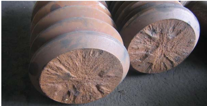
Figure 3. Roll breakage due to too high temperature gradient/high residual stresses.
