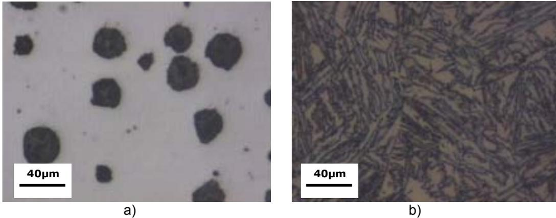
**Figure 4.** Micrography of ADI: a) appearance of graphite in the sample. (without attack); b) appearance of the metallic matrix in the sample (attacked with NITAL 3%).
