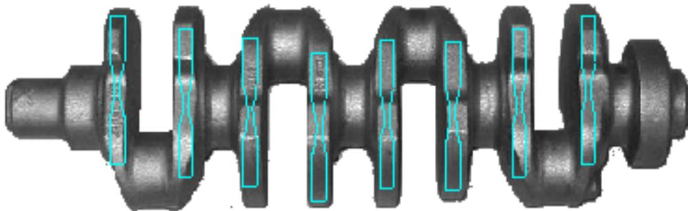
**Figure 1.** Location of the specimens in the crankshaft.
