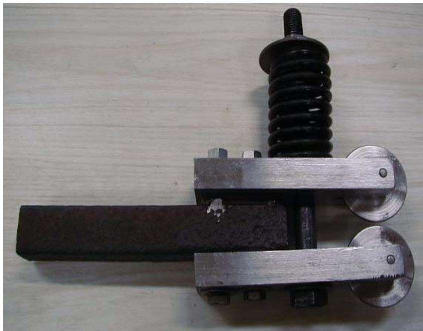
Figure 2. Device for rolling specimens.
