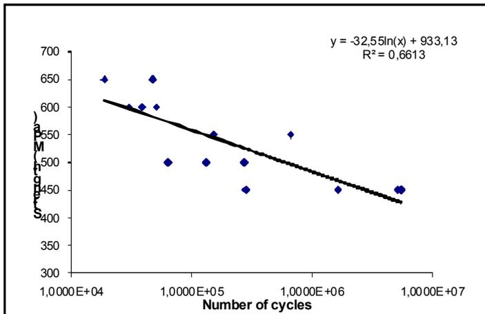
Figure 6. S-N Curve of ADI, submitted to rotational bend with superficial deformation by rolling.
