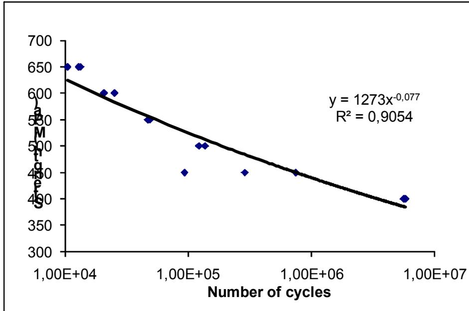
Figure 5. S-N Curve of ADI submitted to rotational bending without superficial deformation.
