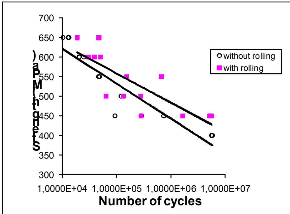
Figure 7. Comparative chart between S-N curves with and without rolling.
