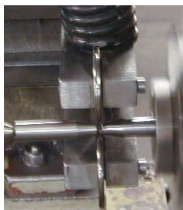
Figure 3. Rolling of specimens in a lathe.
