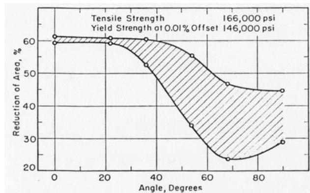
Figure 3: Angle between longitudinal axis and flow direction in specimen to % reduction in area (Wells and Mehl).
