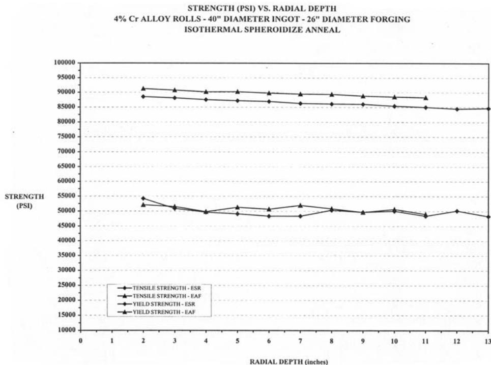
Figure 11: 4% Chromium alloy (EAF\*/ESR) Transverse mechanical properties Tensile strength/yield strength \*Revised practice
