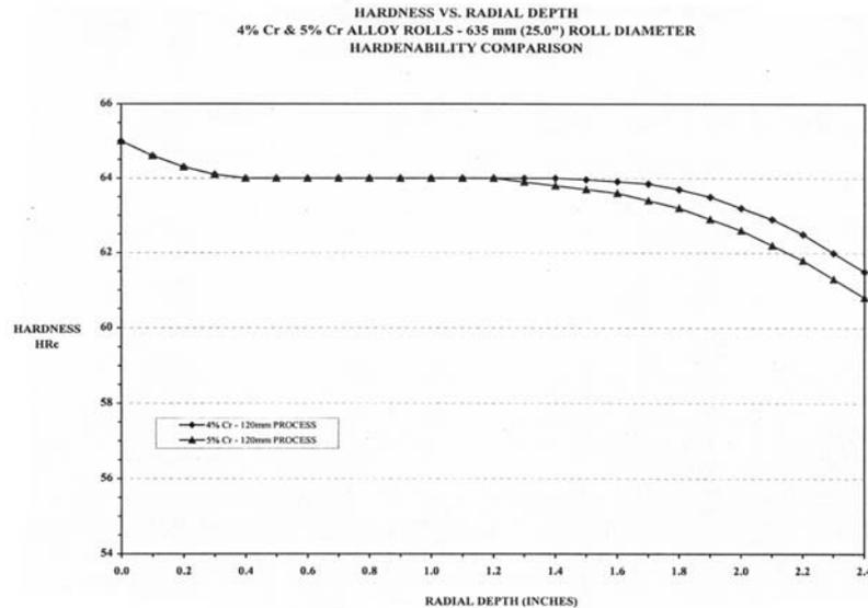
Figure 14: Depth of hardness profiles - 635 mm (25.0 inches) diameter roll (HRc).
