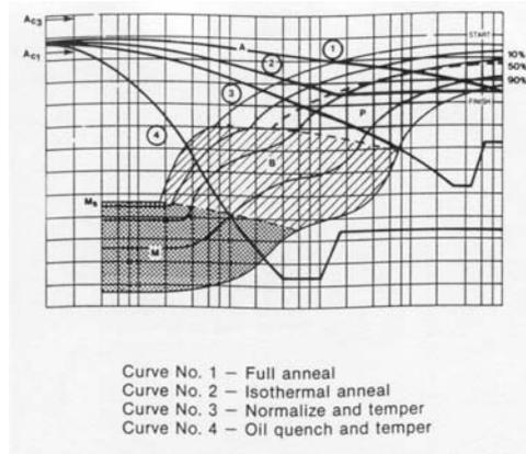
Figure 2: Post-forge heat treatment.
