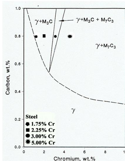
**Figure 1:** Equilibrium phase diagram for the FE-CR-C system at 870° C (1600° F).
