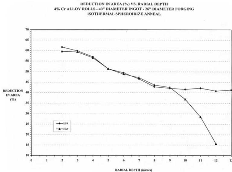
**Figure 9:** 4% Chromium alloy (EAF/ESR) - Transverse mechanical prop. -% reduction of area.
