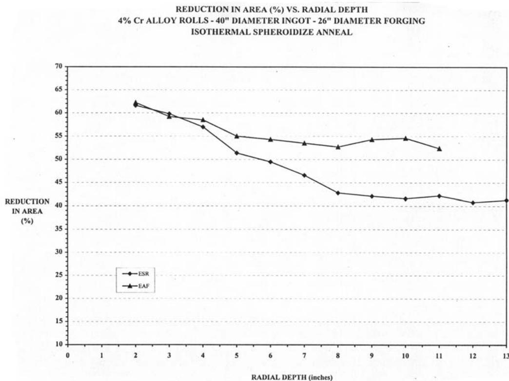
**Figure 13:** 4% Chromium alloy (EAF\*/ESR) Transverse mechanical properties. % Reduction of area
