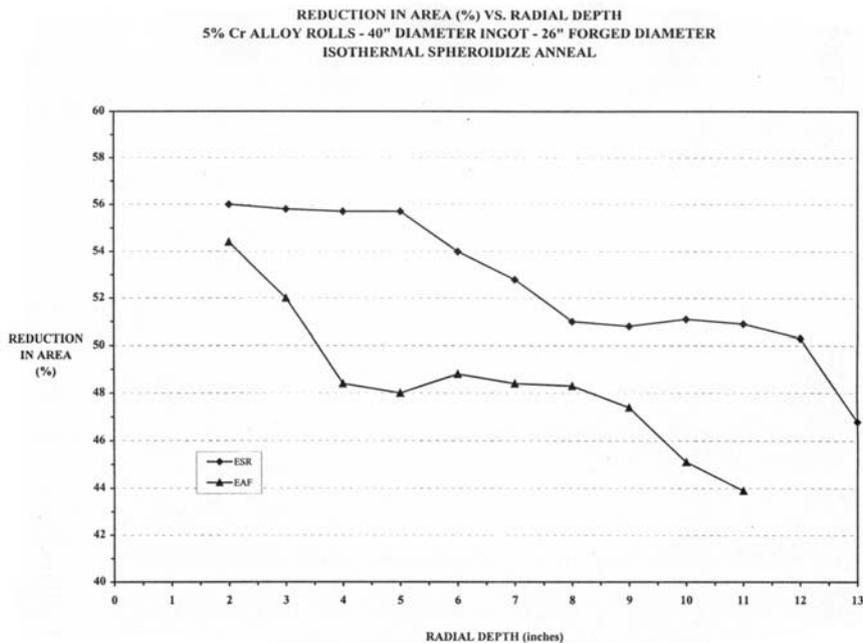
**Figure 6:** 5% Chromium Alloy (EAF/ESR) Transverse mechanical properties % Reduction of area
