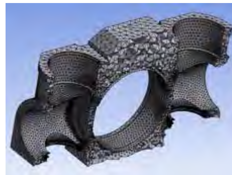
Figure 3. Overall view of the FEM model (200S & 200C).
