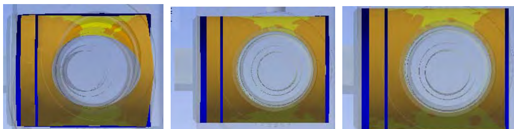
Figure 12. Contact surface (200C) respectively for 100%, 50% and 25 % of the final load.
