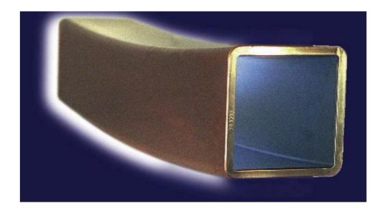
The solution was to design a mold with a highly pronounced taper and with open corner areas in the lower mold zone. This unique mold design thus defines the basis of DIAMOLD technology. The key features are illustrated in below figure and can be summarized as follows:
