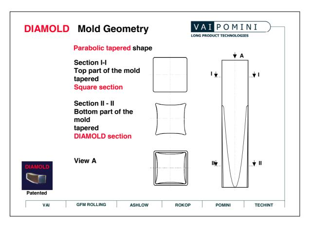
Before mentioned design criteria result in Casting Speed which are up to 50% higher than with standard conicities, it allows for a very wide operating window, covering a wide range of different steel grades with different shrinking behavior and casting speed.
