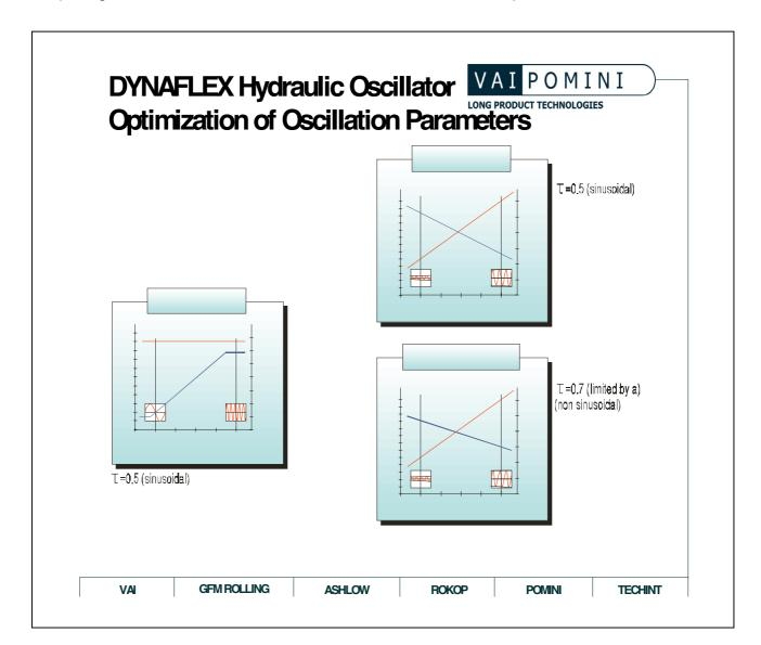
The advantages of the modern actuator mechanism permit the achievement of ideal oscillation characteristics (figure above), as the waveform (sinusoidal, non-sinusoidal, saw-curve, etc.), stroke (amplitude) and frequency (strokes per minute) can be varied in order to optimize the positive and negative strip time as desired:
