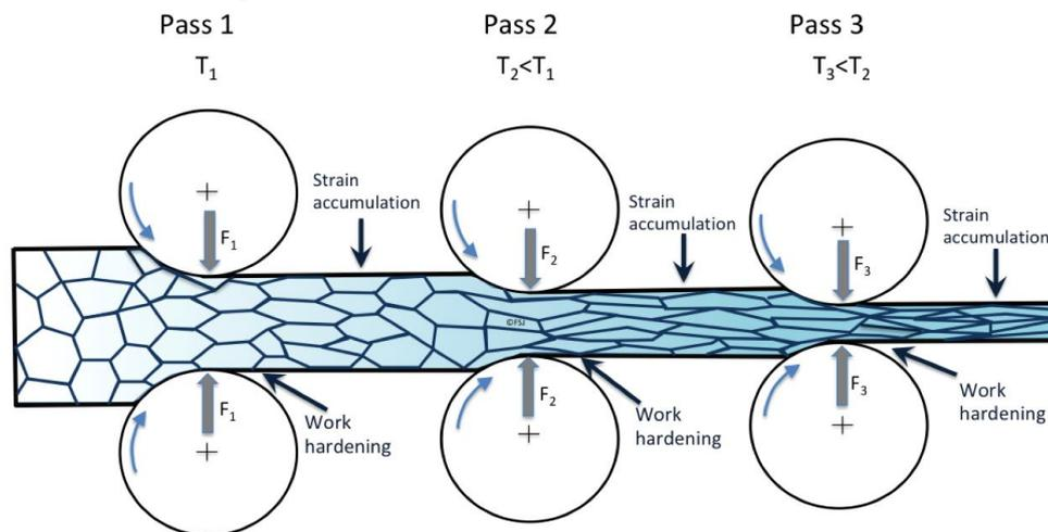
Figure 3. Schematic representation of the microstructure evolution during the conventional controlled rolling process [18].
