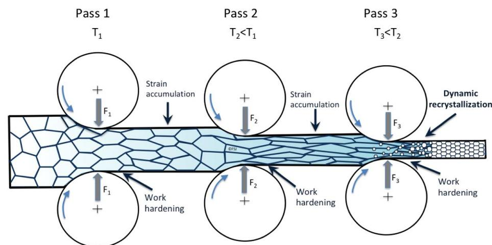
Figure 4. Schematic representation of the microstructure evolution during the dynamic recrystallization controlled rolling process [18].
