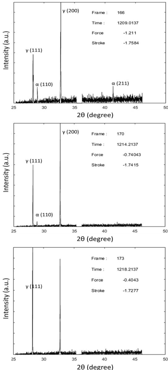
Figure 7. X-ray spectrum patterns taken (a) during final stage of deformation (b) 5 seconds after unloading and (c) 9 seconds after unloading.
