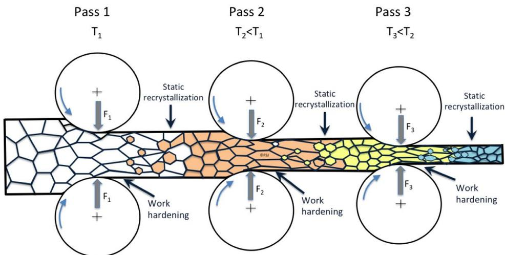
Figure 2. Schematic representation of the microstructure evolution during the recrystallization controlled rolling process [18].
