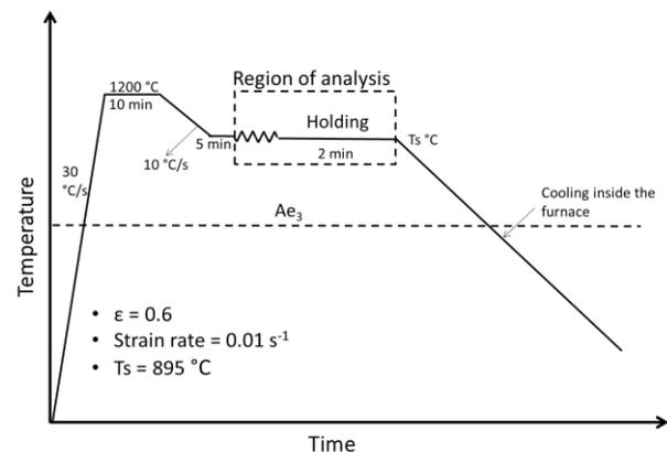
FIGURE 6. Test schedule of the compression samples of microalloyed steel.
