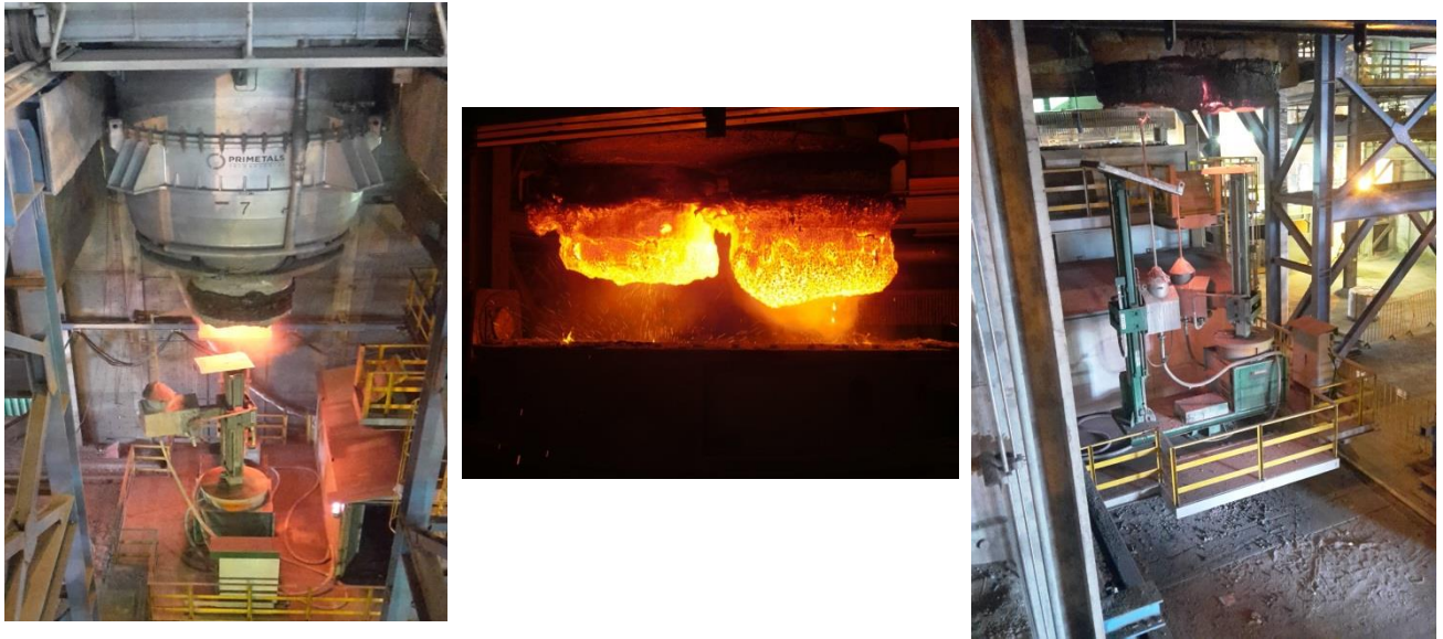
Figure 9 Snorkel gunning machine in operation
