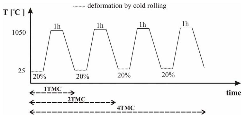
**Figure 1.** Schematic representation of the thermomechanical processing procedure used in this work.<sup>(21)</sup>
