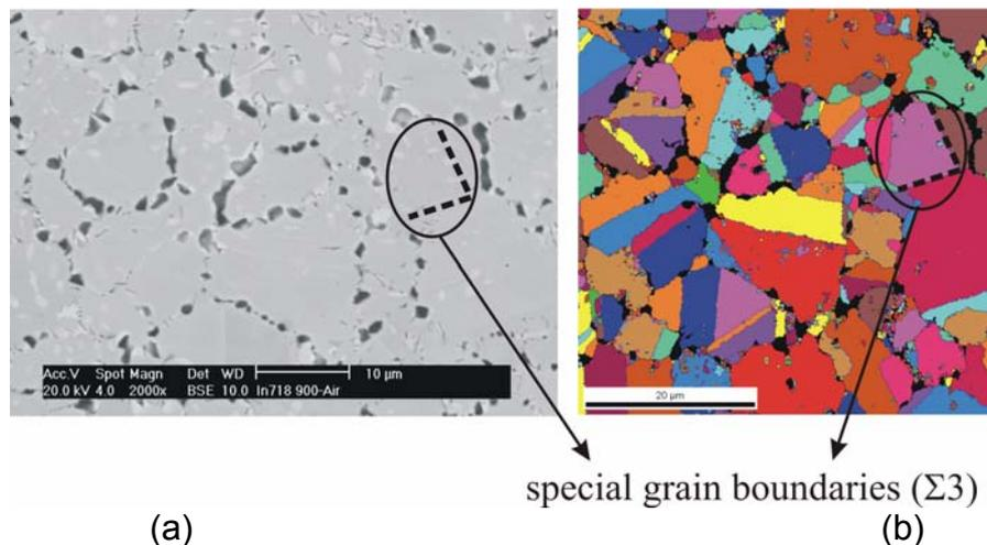
**Figure 5.** Analysis of the surface (the external  $\text{Cr}_2\text{O}_3$  scale was removed) of an oxidised specimen in laboratory air at  $850^\circ\text{C}$ : (a) grain boundary structures and (b) oxide formation along random grain boundaries.<sup>(25)</sup>
