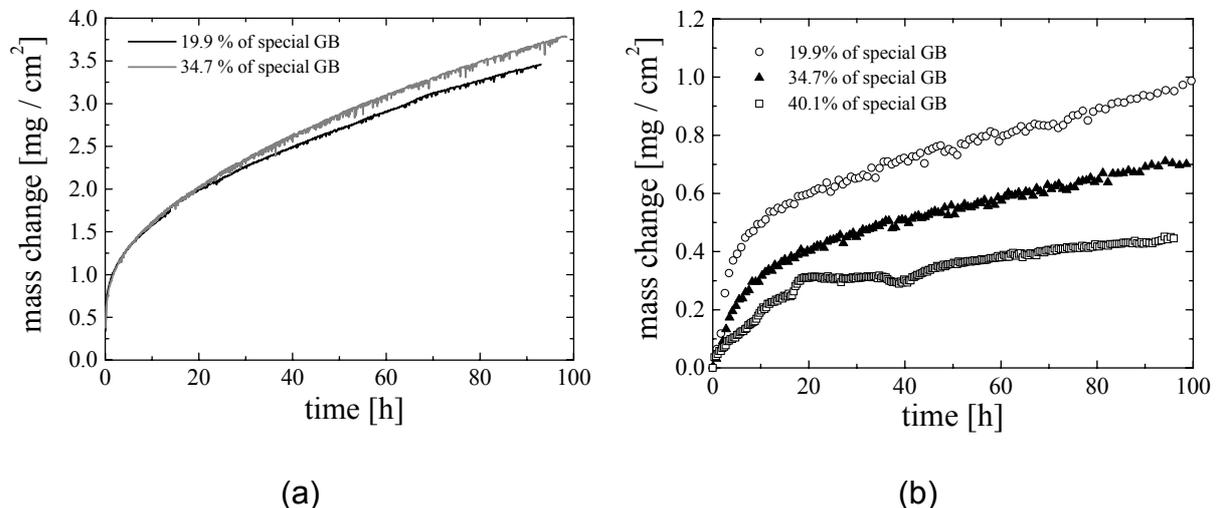
**Figure 3.** Thermogravimetrically measured mass change during exposure of IN718 to laboratory air for different fractions of special grain boundaries: (a) at 1000°C and (b) at 850°C. <sup>(21)</sup>
