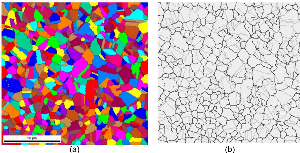
**Figure 1.** (a) Orientation map and (b) CSL grain boundary distribution (special grain boundaries are marked as gray lines).<sup>(21)</sup>
