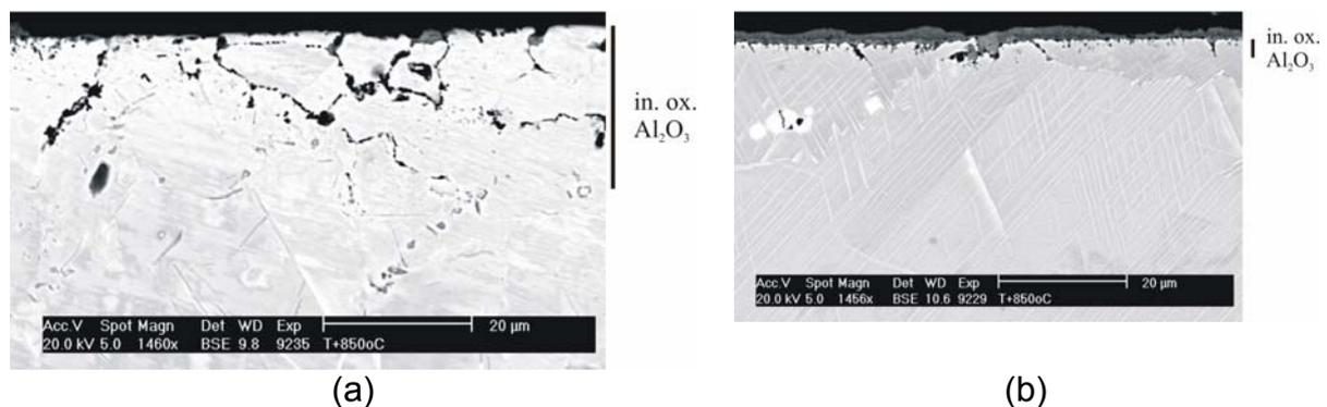
**Figure 4.** SEM-cross-section micrographs of the intergranular oxidation zone (in. ox. Al<sub>2</sub>O<sub>3</sub>) in IN718 oxidised in laboratory air at 850°C: (a) 1TMC\* and (b) 4TMC (white areas correspond to  $\delta$  phase). \* Spallation of the outer oxide scale occurred during preparation.
