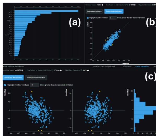
Figure 4: (a) Variable Impact and residual analysis, (b) LR Predicted vs, LR Actual and (c) Residues Analysis for the expanded LR Model.
