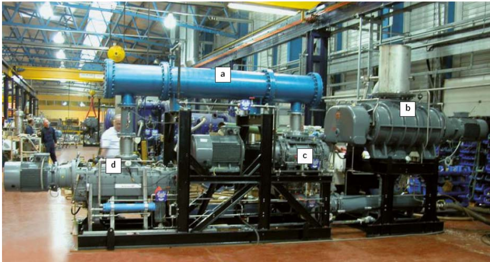
Figure 4. Skid configuration of the vacuum pump. (a) Heat exchanger; (b) HV pump; (c) SN pump; and (d) IDX pump.
