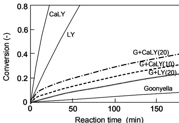
**Figure 11.** Time-conversion curves for various cokes during CO<sub>2</sub> gasification (CO<sub>2</sub>/N<sub>2</sub>-50/50, 1000°C).
