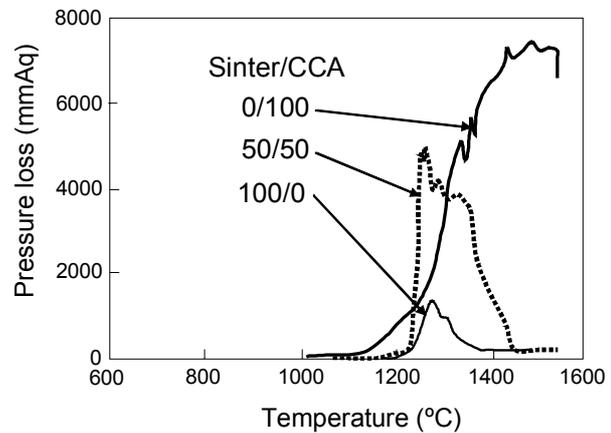
**Figure 14.** Changes of gas pressure drop of iron ore bed by mixing the carbon composite iron ore.
