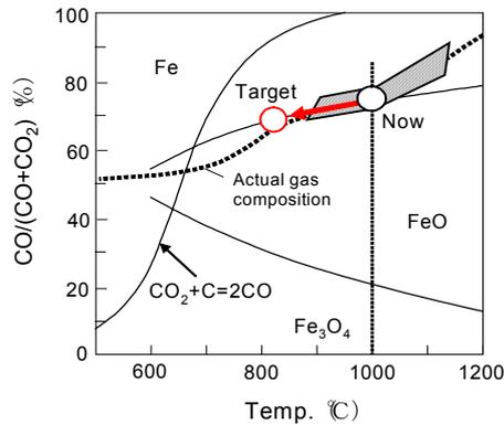
**Figure 3.** Gas composition in actual blast furnace.
