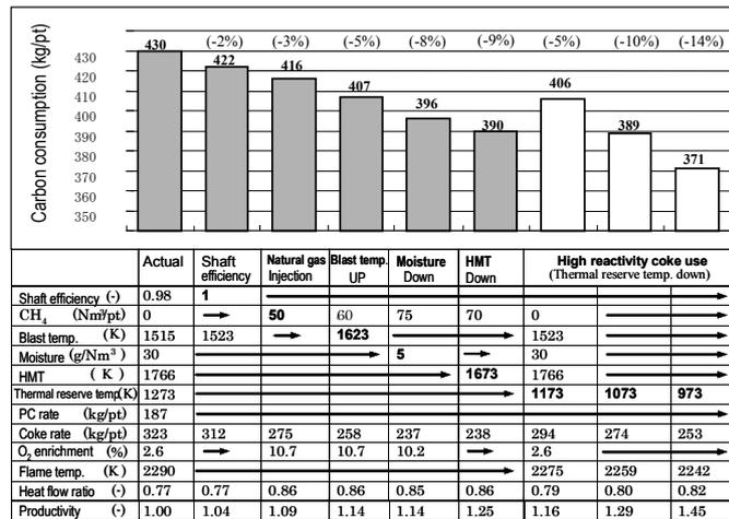
**Figure 4.** Effect of operation condition on coke rate and productivity by Rist diagram.
