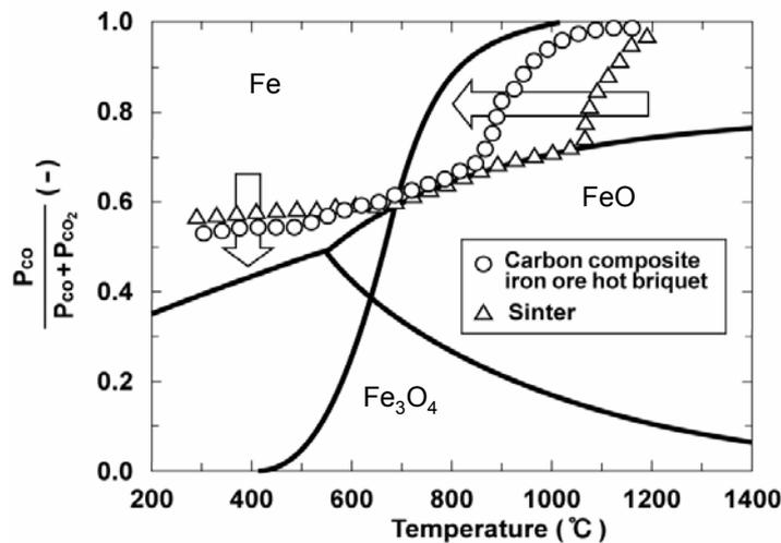
**Figure 9.** Change of reduction reaction equilibrium at charging of CCB in model blast furnace test.
