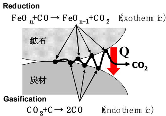
**Figure 7.** Coupling reaction effect between reduction of iron oxide and Boudouard reaction.
