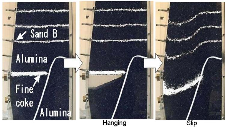
**Figure 12.** Hanging and slip caused by formation of impermeable layer in the lower part of blast furnace.
