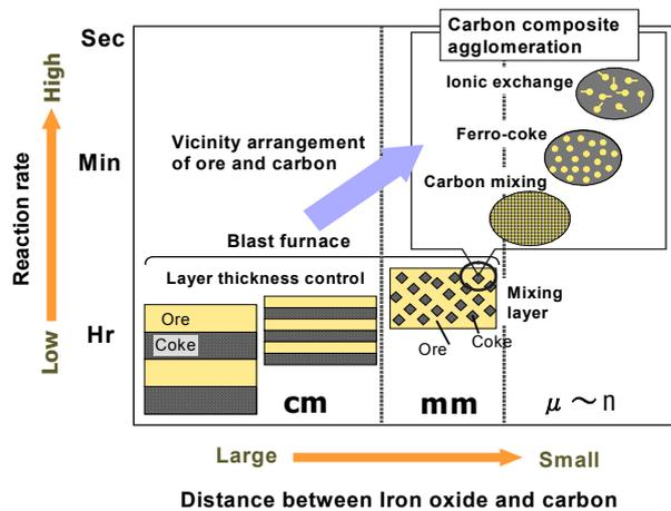
**Figure 5.** Relationship between reaction rate and arrangement of iron oxide and carbon.
