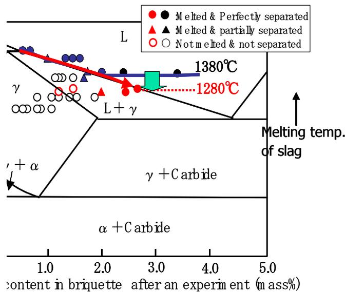
Figure 15. Melting temperature of carbon composite iron ore briquette.
