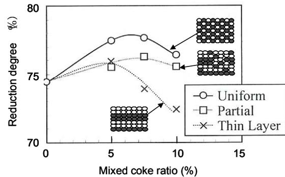
**Figure 6.** Change in reduction degree by mixed coke with mixing way at 1200°C.
