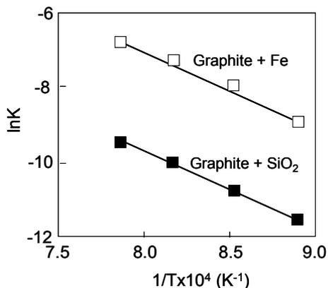
**Figure 10.** Effect of Fe addition on the gasification rate of graphite in 20% CO<sub>2</sub>-CO mixture.
