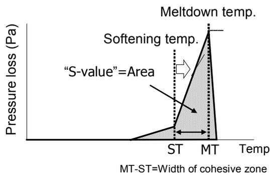
**Figure 13.** Change of gas pressure loss in softening and melting of iron ore bed.
