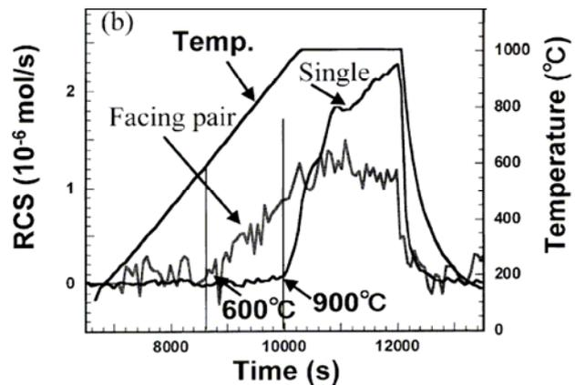
**Figure 8.** Comparison of reaction rate between the facing pair and the single graphite in Ar-30vol%CO<sub>2</sub>.
