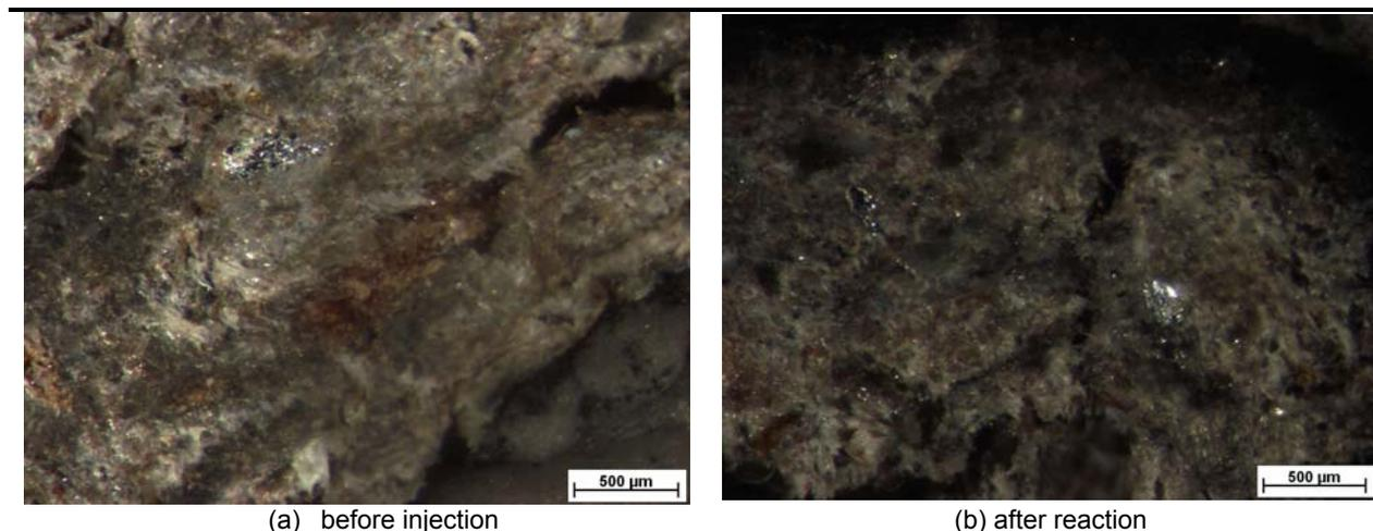
**Figure 10.** Surface cut of an agglomerate particle before and after the injection.
