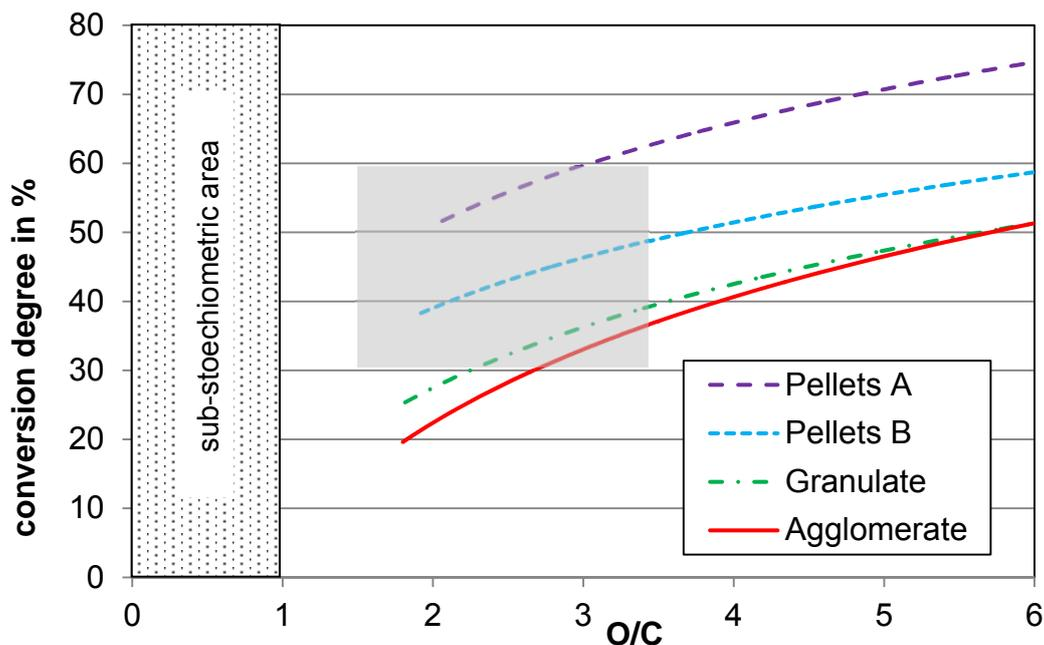
**Figure 8.** Conversion degree against O/C atomic ratio for the 4 types of waste plastics.
