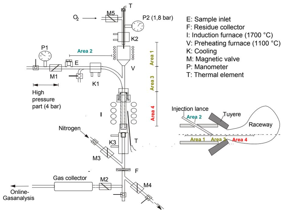
Figure 7. Scheme of the Batch Injection Rig at the IEHK.<sup>(12)</sup>
