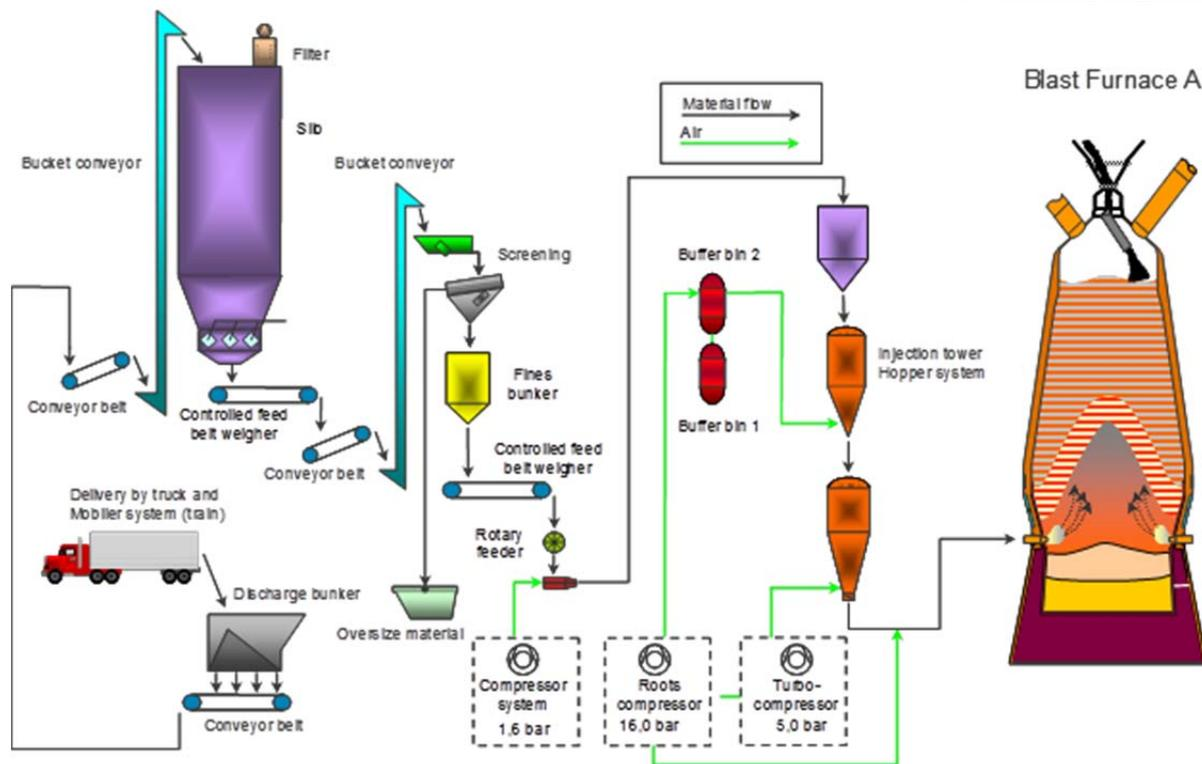
Figure 1. Layout of plastics injection at voestalpine Stahl BF A.
