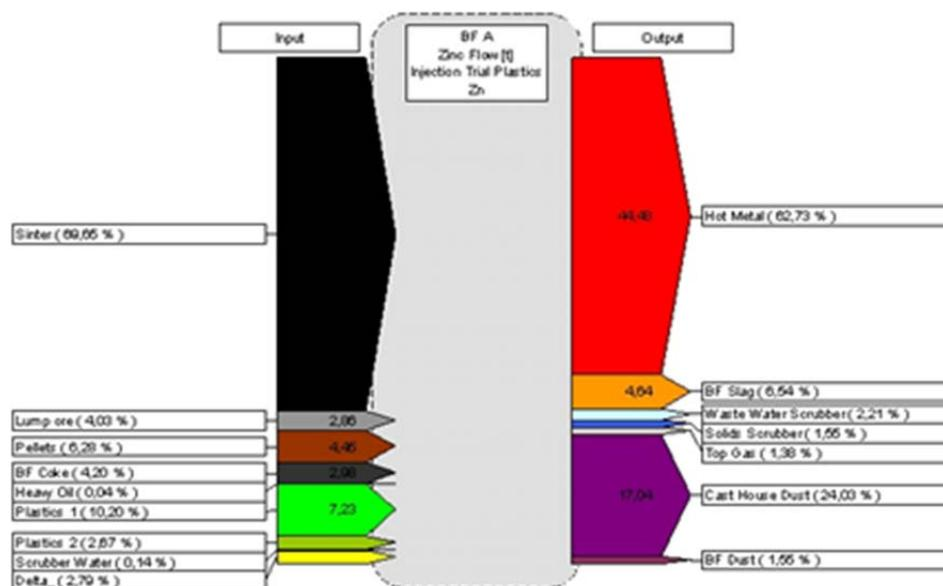
Figure 3. Substance flow analysis Zn for BF process with secondary raw materials.
