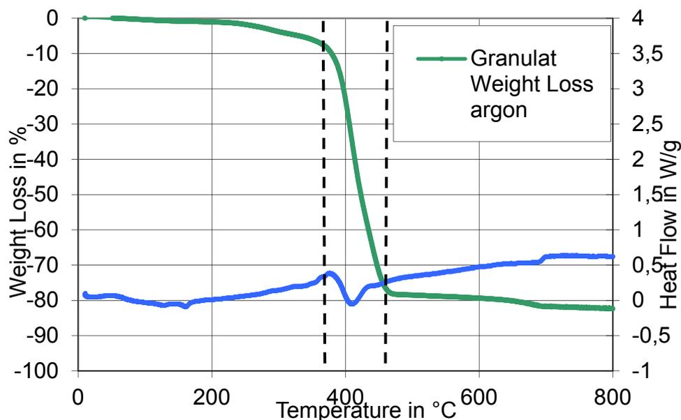
**Figure 5.** Specific weight loss and heat flow of granulate in argon atmosphere.
