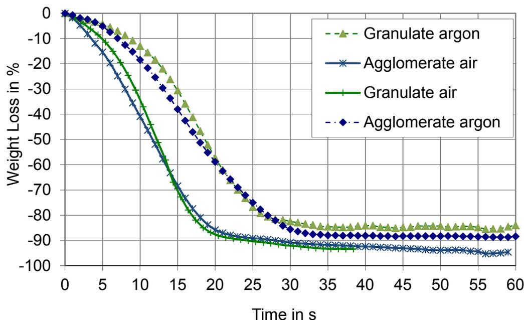
**Figure 6.** Weight loss of waste plastics in argon atmosphere.
