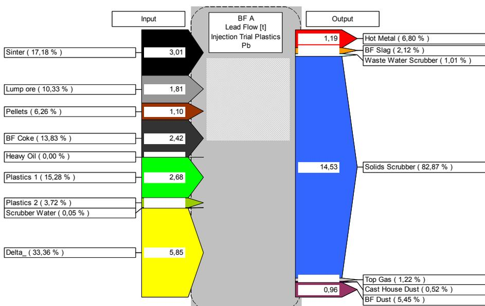
Figure 4. Substance flow analysis Pb for BF process with secondary raw materials.
