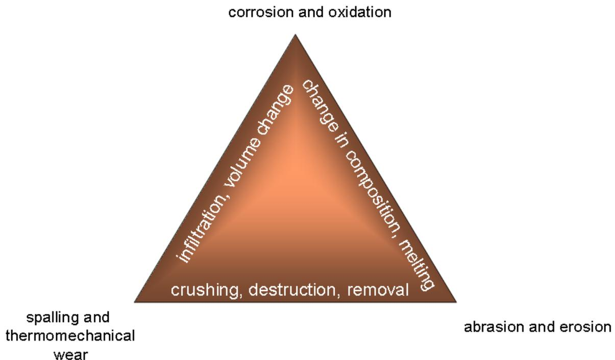
Figure 1: Triangle of refractory wear in a BOF.
