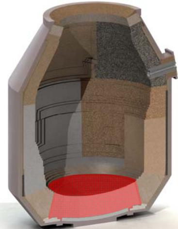
Figure 12: Bottom in a BOF-lining.
