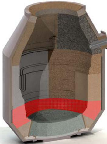
Figure 11: Lower Cone in a BOF-lining.
