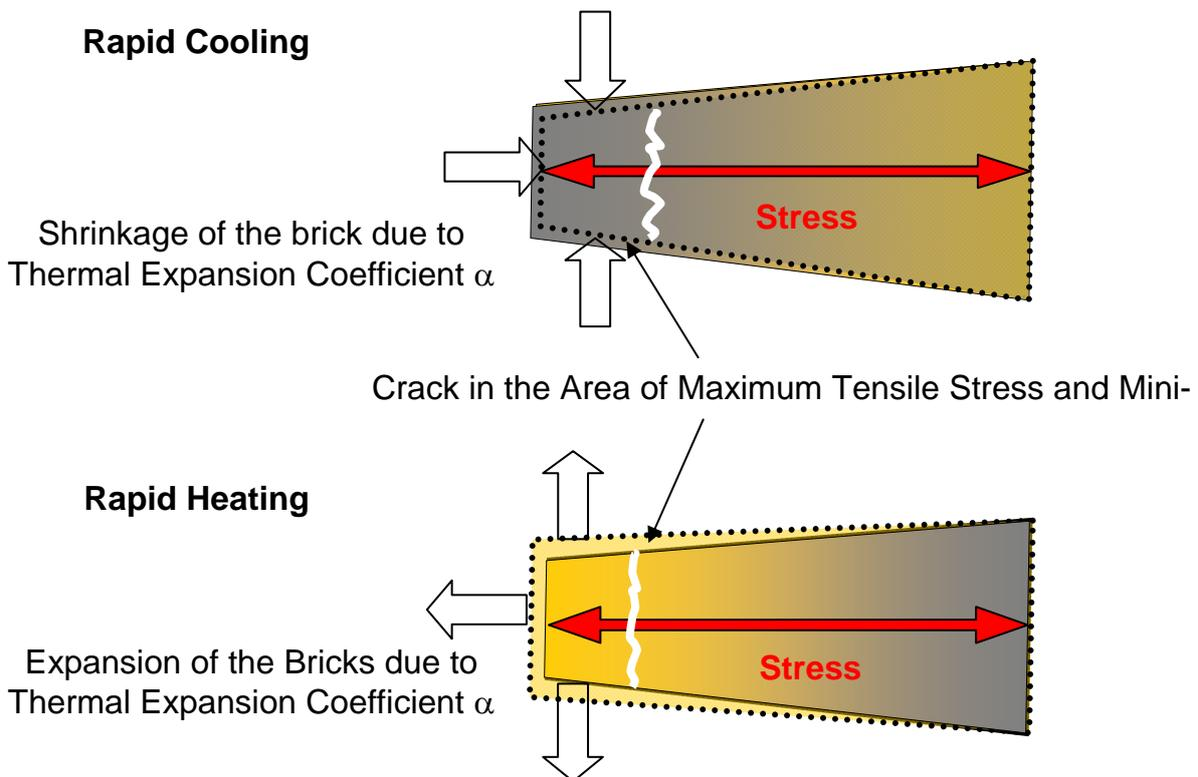
Figure 13: Crack formation in MgO-C bricks through thermal cycling.
