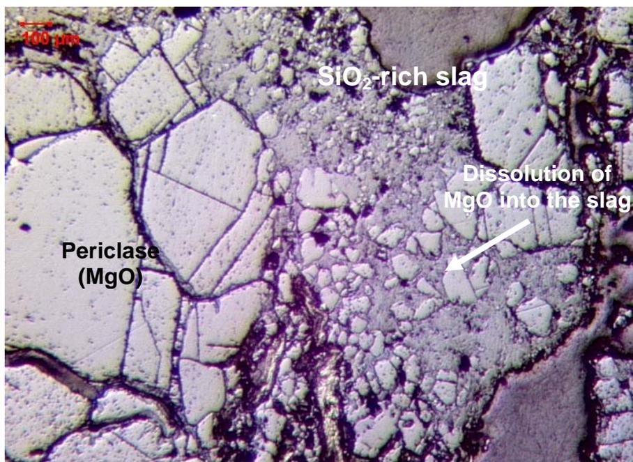
**Figure 10:** Microphoto of an MgO-C brick with corrosion attack by SiO<sub>2</sub>-rich slags.
