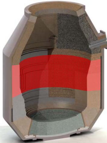
Figure 2: Barrel in a BOF-lining.
