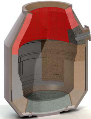
Figure 3: Upper Cone in a BOF-lining.
