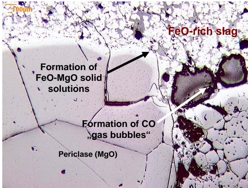
**Figure 6:** Microphoto of an MgO-C brick with severe corrosion attack by FeO.
