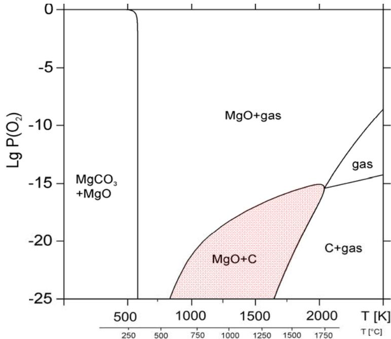
Figure 4: Temperature -  $p(O_2)$  - Diagram of MgO-C.
