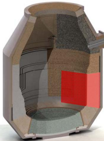
Figure 14. Scrap Impact in a BOF-lining
