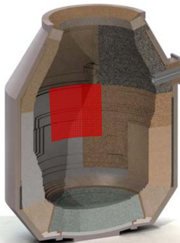
**Figure 7:** Trunnion in a BOF-lining.
