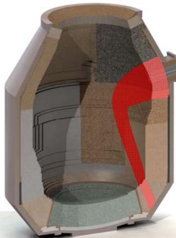
Figure 5: Tapping Zone in a BOF-lining.
