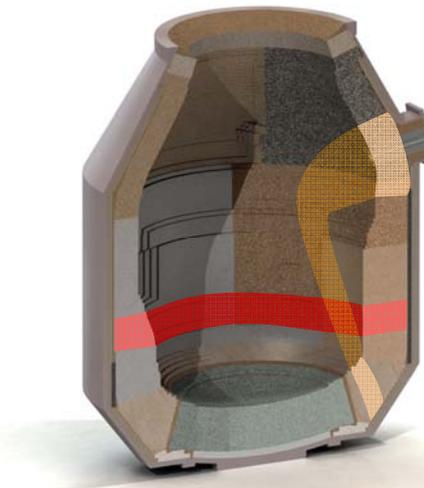
**Figure 8:** Slag Zone (red) and intersection ("slag-cross") with Tapping Zone (yellow, see Fig. 5) in a BOF-lining.
