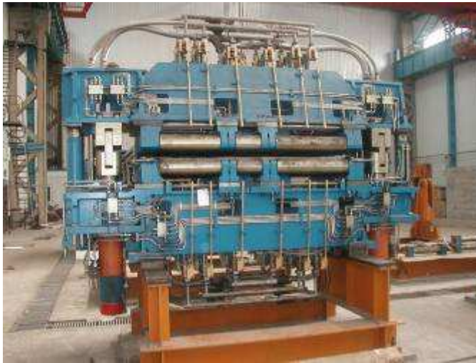
Figure 3 : Danieli segments with split roll design and air mist secondary cooling
