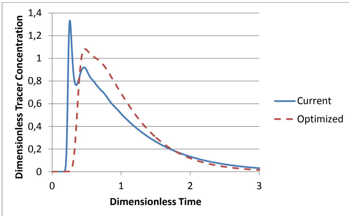
Figure 11: Comparison between the obtained RTD Curves for the reference case and the optimized weir and dam configuration.
