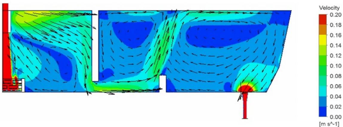
Figure 3: Flow Pattern with large recirculation zones behind the weir and the dam.
