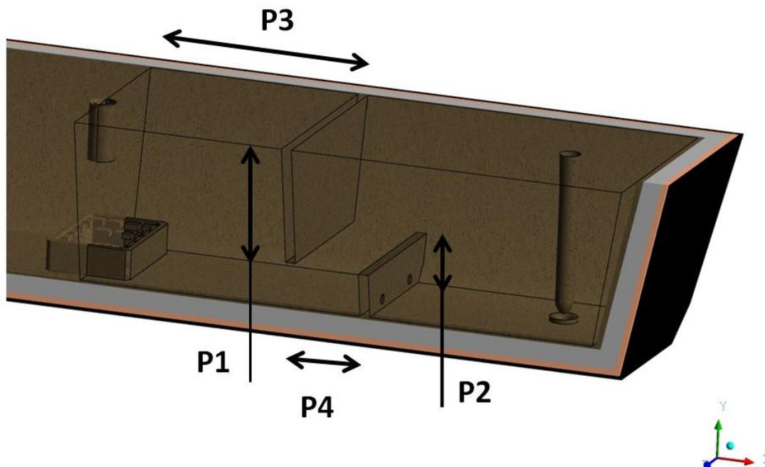
Figure 5: Optimized parameters of the weir and dam configuration.
