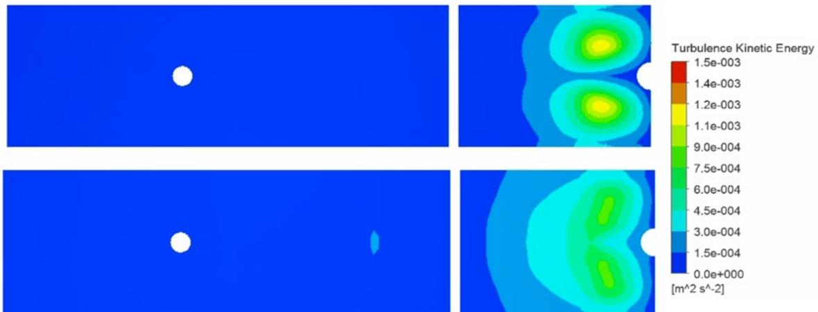
Figure 9: Comparison between the turbulence kinetic energy at the slag surface for the reference case and Candidate 03 proposed by the optimization.
