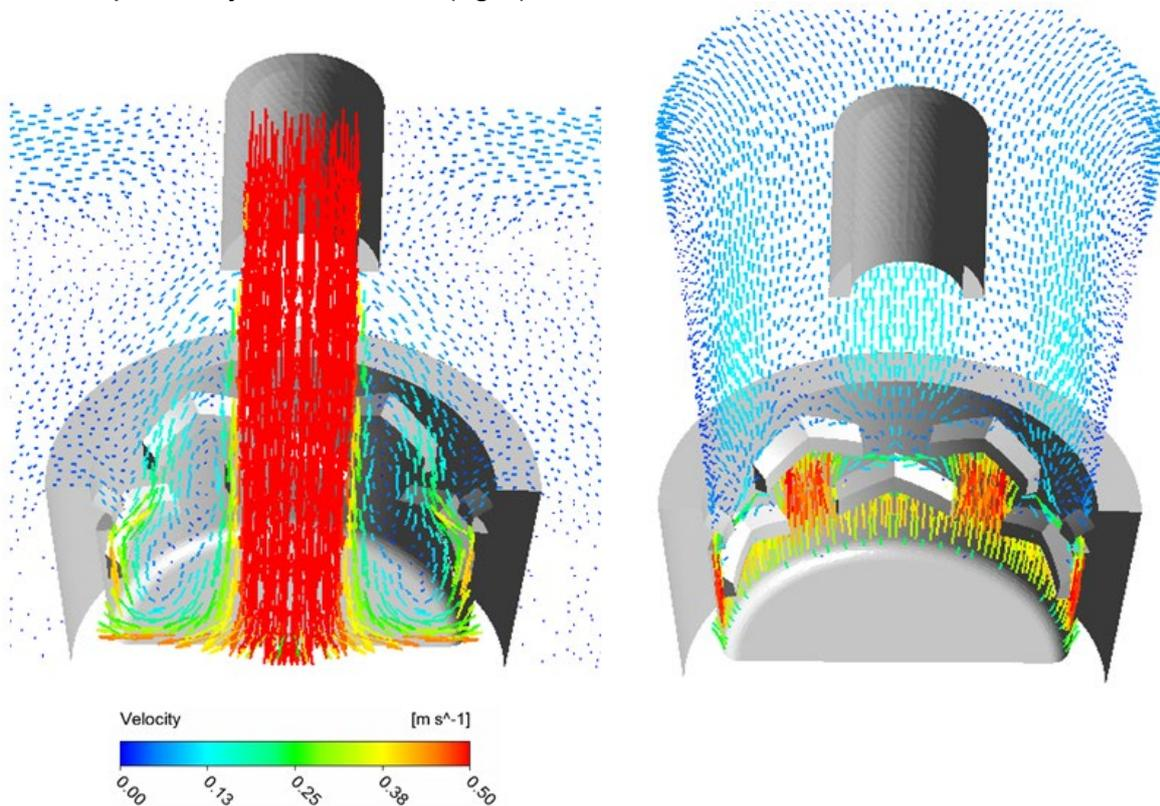
Figure 2: Entry jet's kinetic energy dissipation by a TUNFLOW Chevron™.
