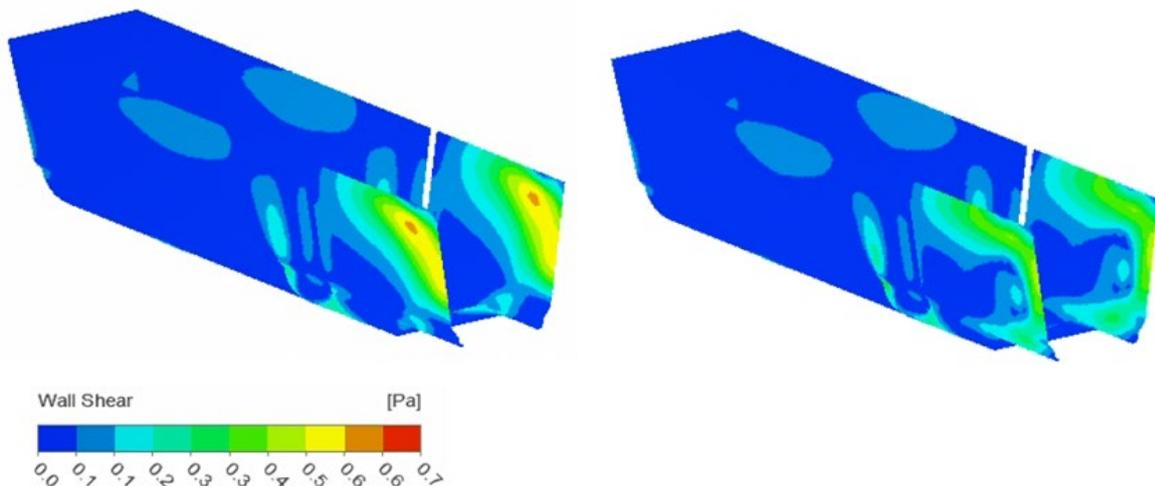
Figure 7: Comparison between wall shear stresses of the reference case (left) and Candidate 01 proposed by the optimization model (right).
