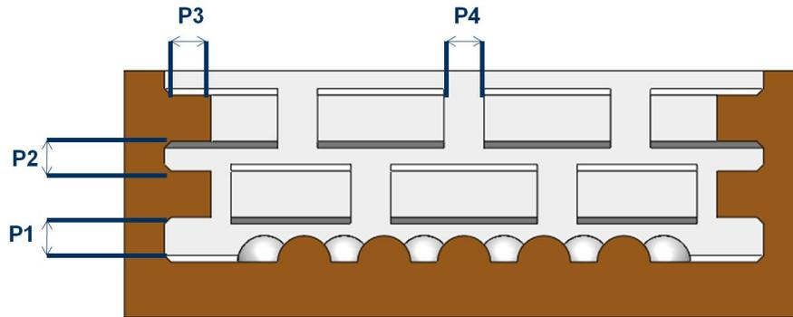
Figure 4: Optimized parameters of the RisalImpact<sup>™</sup> geometry.
