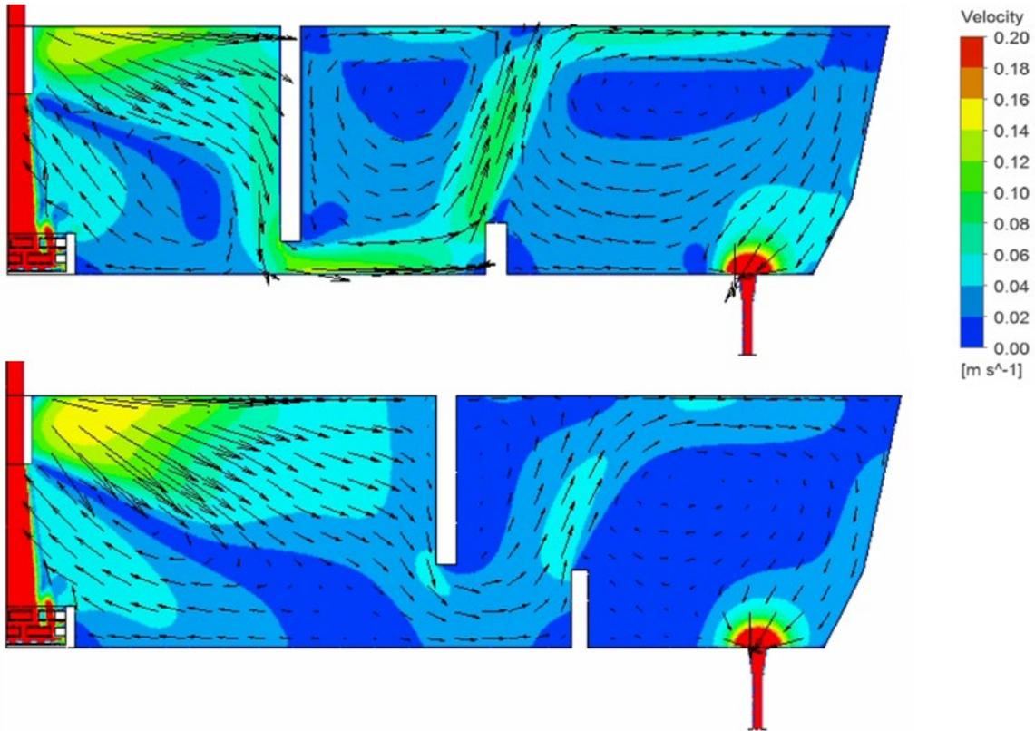
Figure 10: Comparison between the obtained flow patterns for the reference case (above) and optimized weir and dam (below).
