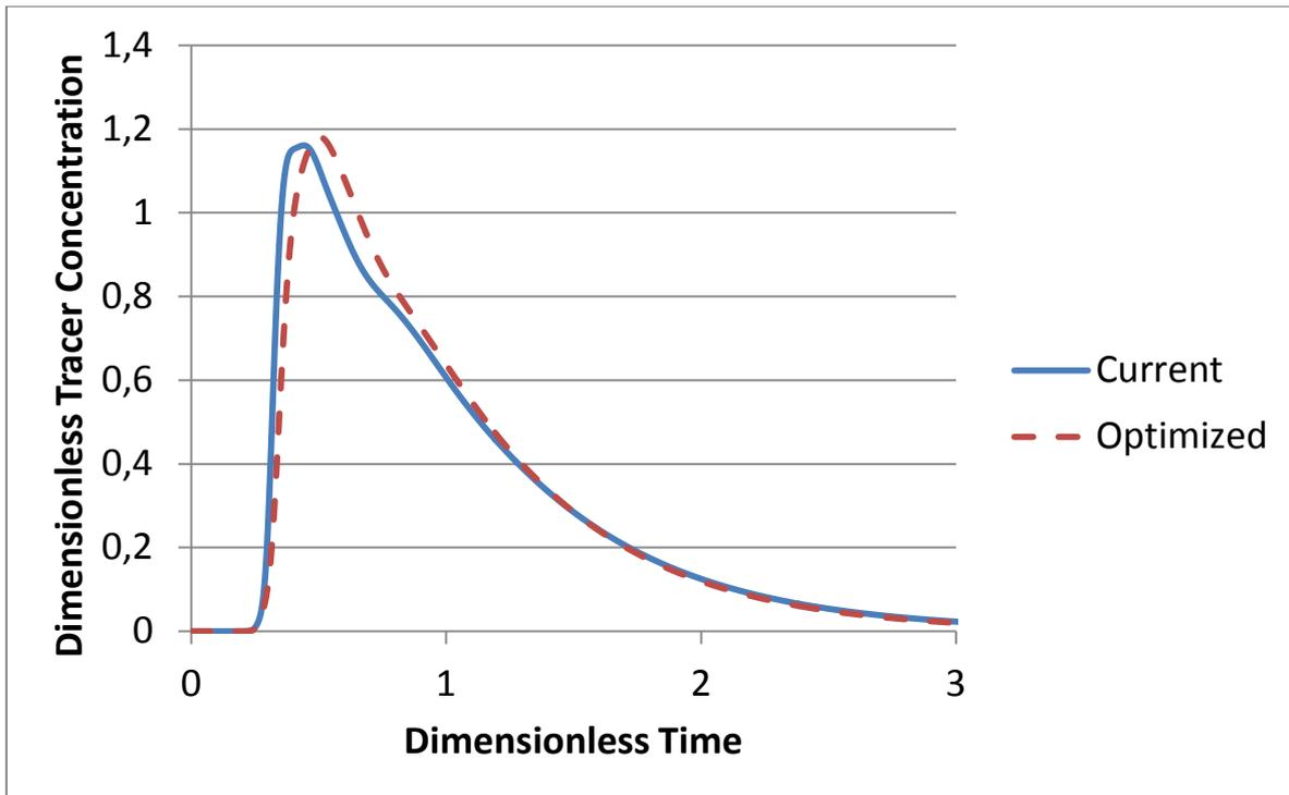
Figure 8: Comparison between the obtained RTD curves for the current case and Candidate 02 proposed by the optimization.
