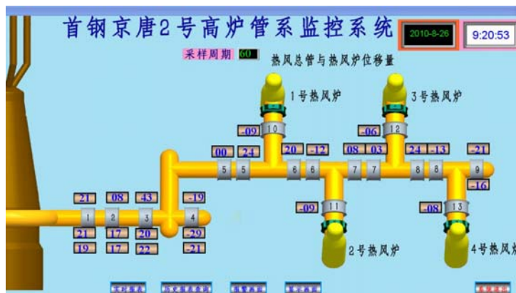
Figure 5 Deformation monitoring interface.
