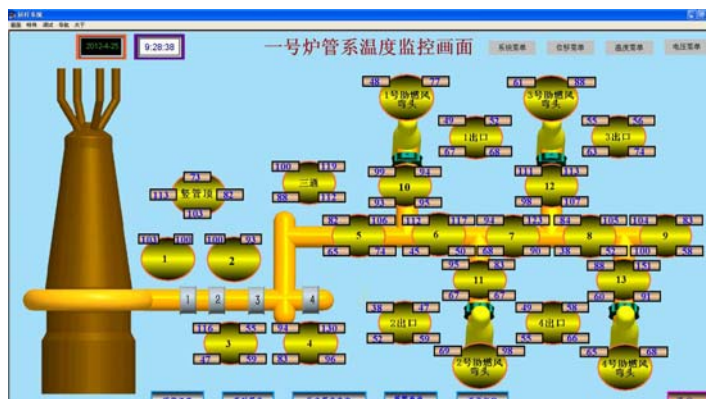
Figure 3 Pipelines temperature interface.
