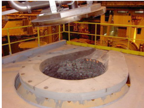
Figure 4: Spout design for “monoblock”
