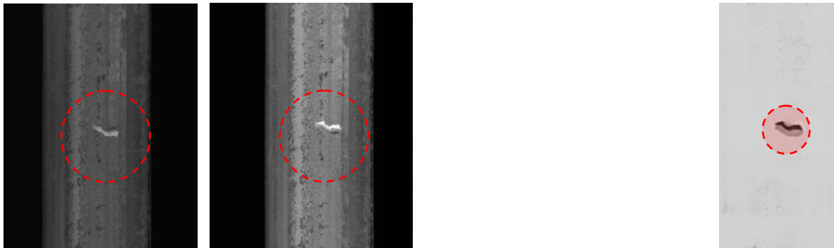
Figure 2. (left) Different directions of light, “different” images of the same defect
