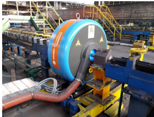
Figure 1. Installation of a HiNSPECT wire rod application
