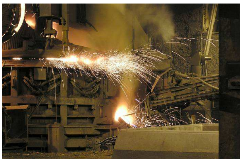
Figure 1: Celsa Armeringsstål EAF before revamping with the door manipulator.
