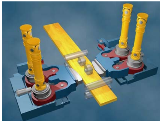
Figure 2: Functional principle of the slab sizing press.
