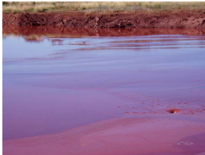
Figure 10: Initial paste deposition – note depression indicating yield stress
