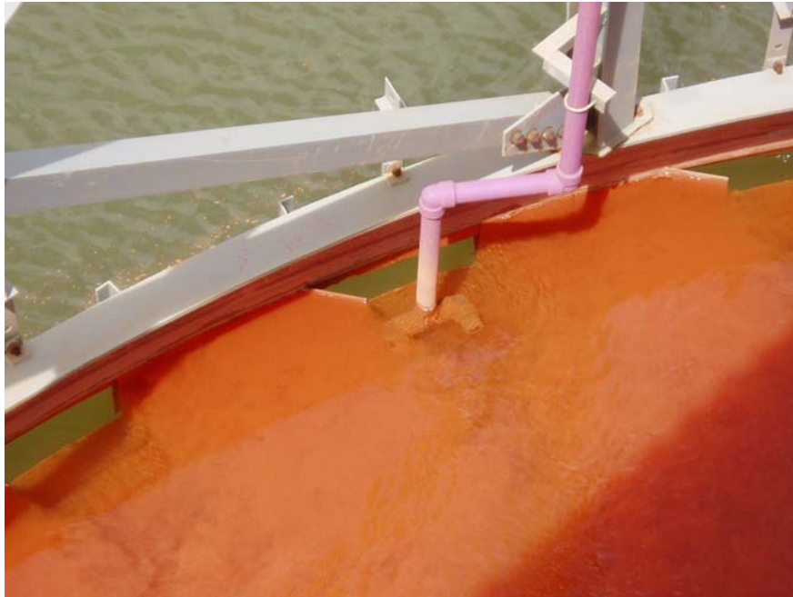
Figure 6: Feedwell showing supernatant dilutant flowing through a port, past the flocculant nozzle
