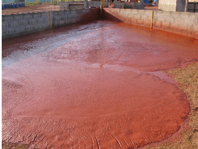
Figure 4: Flume testing to determine deposition slope
