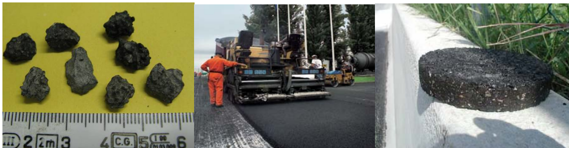
Figure 10. Ecogavel®; Road application; and a sample of the final product bituminous conglomerate.
