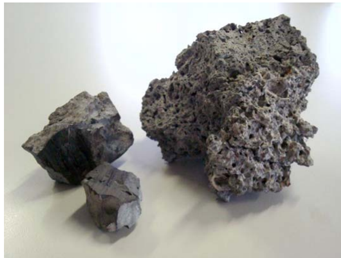
Figure 3. Compact and porous EAF slag.
