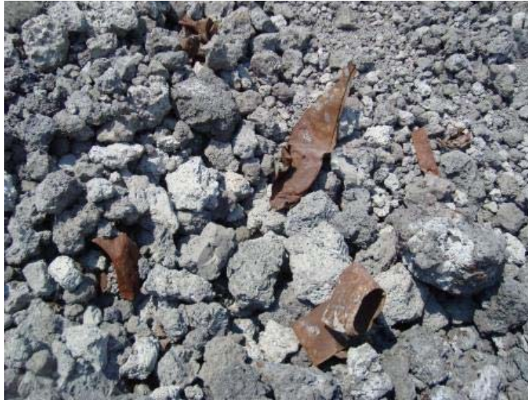
Figure 8. Recoverable scrap within the slag.
