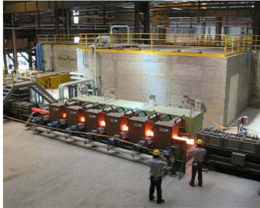
Figure 3: Induction heating system in operation.
